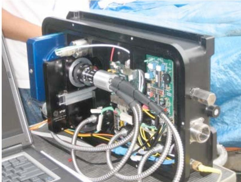
Fig. 3.3 Image of the interior of the polarization camera system. On the far left is the camera (the blue box), in front of which is the IFW filter chamber. The coherent fiber bundle is shown, with each leg going to fisheye lenses in the lower portion of the box. We also have a pressure transducer, tilt and roll indicator, and other associated electronics. The system is controlled by the laptop shown on the left of the picture.
