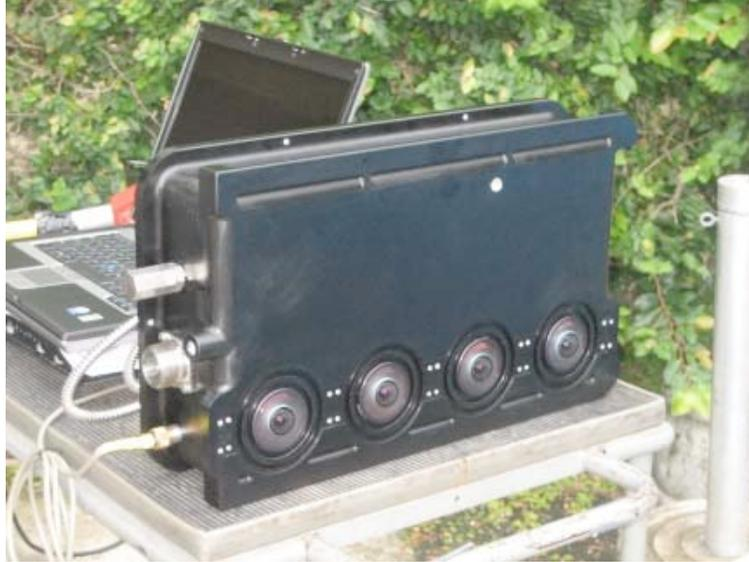
Fig. 3.2 Image of the top of the polarization camera system. One can see the four fisheye lenses all aligned in a row. On the left are connectors to allow the system to be used either over a dedicated cable (the big connector) and fiber, or through a copper ethernet connection.
