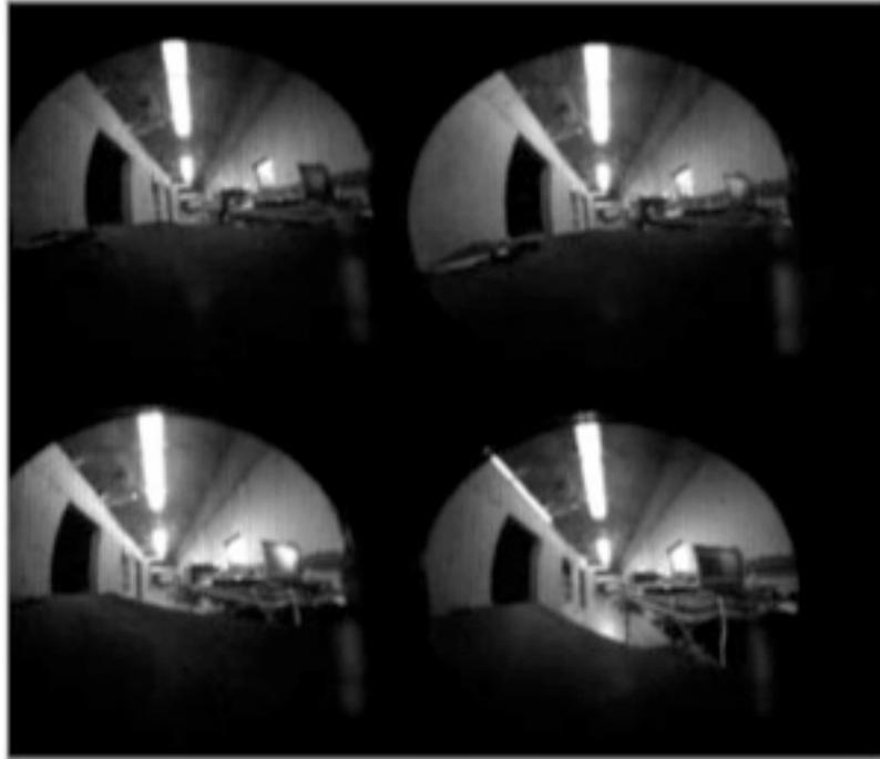
Fig. 3.1 Sample image from DPOL camera system. There are 4 separate fisheye images shown in this one camera image, the result of our quadfricated fiber bundle. Each small fisheye image carries different polarization information. Three of the images have linear polarizers in line with the image optical path. The remaining image contains a circular polarization analyzer. By combining these images, the 4 Stokes parameters can be determined.
