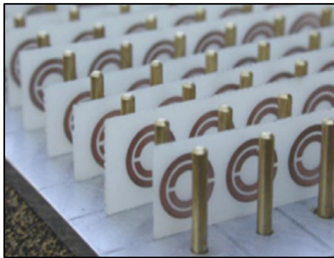
Figure (3.1): First experimental monodimensionally LHM structures consisted of thin continuous wires and SRRs (Pandey, et al.).
