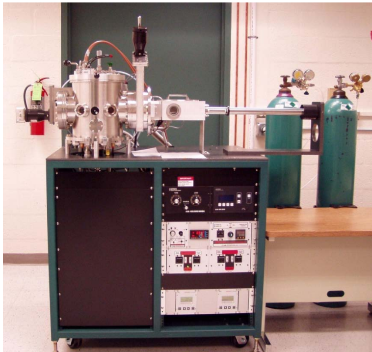
Figure 4.2. Picture of our magnetron sputtering, notice the load lock
