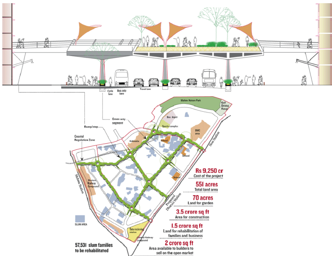
Figure 3.4 Proposed plan of the Dharavi Redevelopment BMC Project and projection of the allotted acreage
