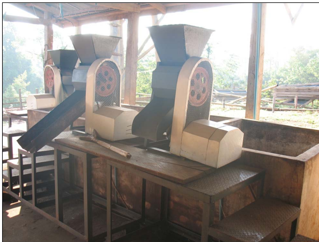
Image 12: An PCADR-PAB-sponsored wet-processing station in a Bolaven Plateau village ( Ban 38 Kapeu) with an active AGPC producers' group. Source: Photograph by author, March 20, 2009.
