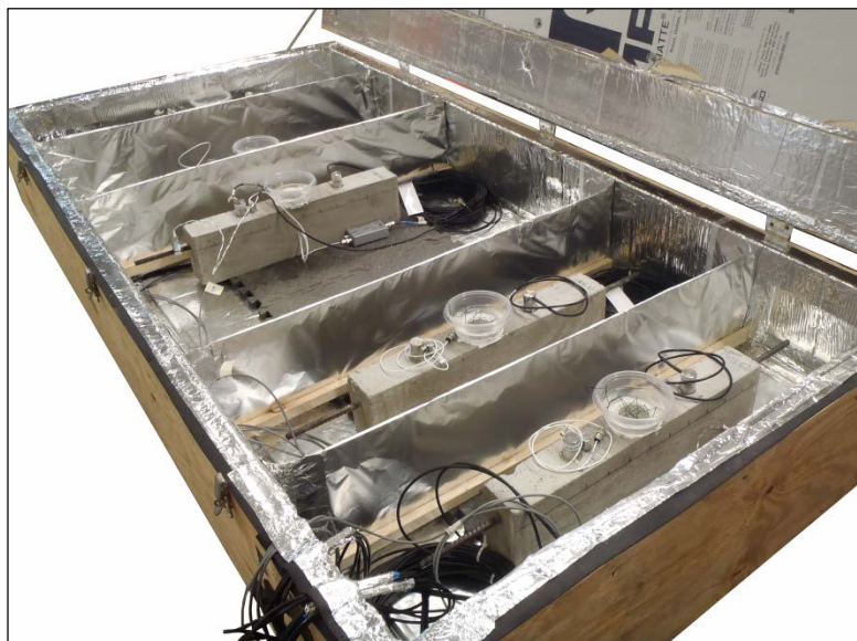
Figure A.28 – Accelerated corrosion test setup
