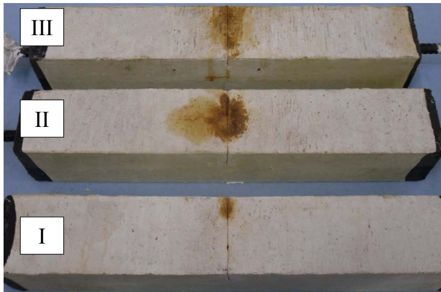
Figure A.21 – Specimens 0.2 mm - #2 after accelerated corrosion test
