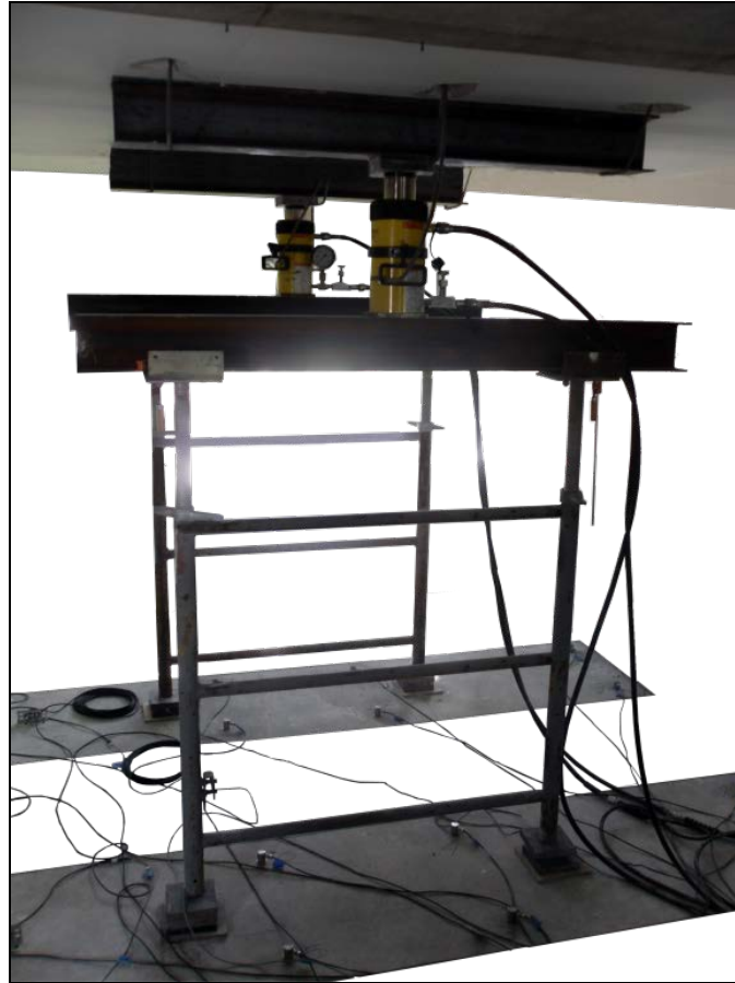
Figure 19 – Load test setup
