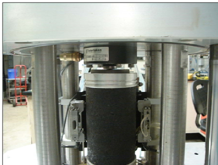
Figure A30 Lifting of the sample until it touches top
