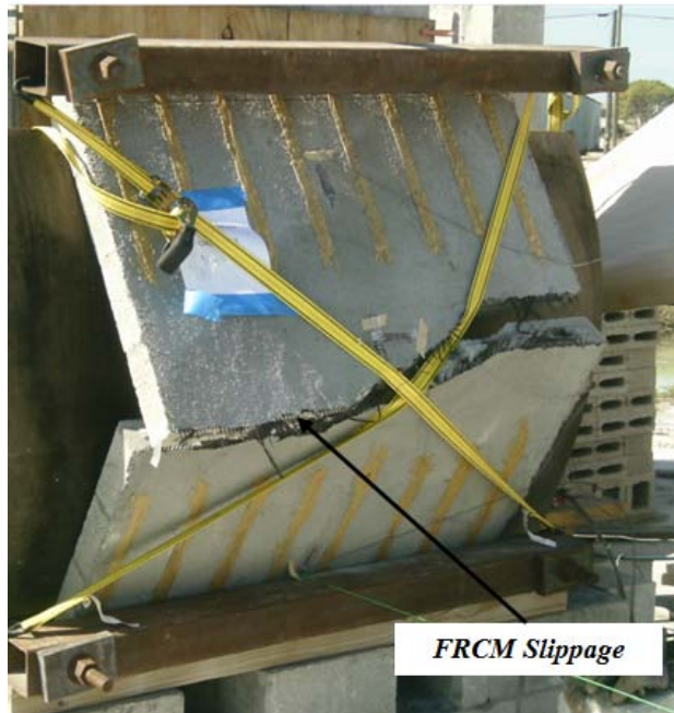
(b) (Fabric breaks because of collapse)
