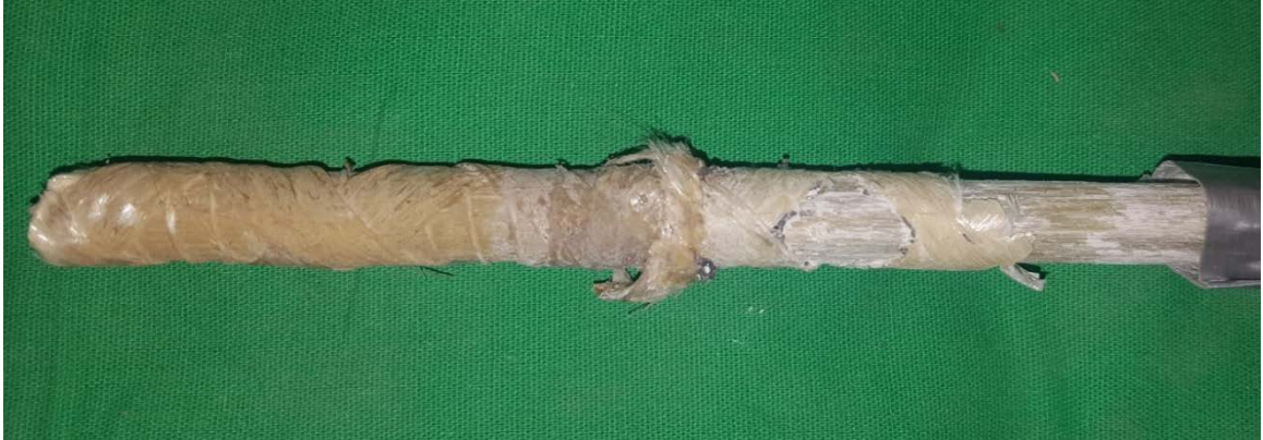
Fig. 7 Detail of the extracted GFRP bar after pull out test.
