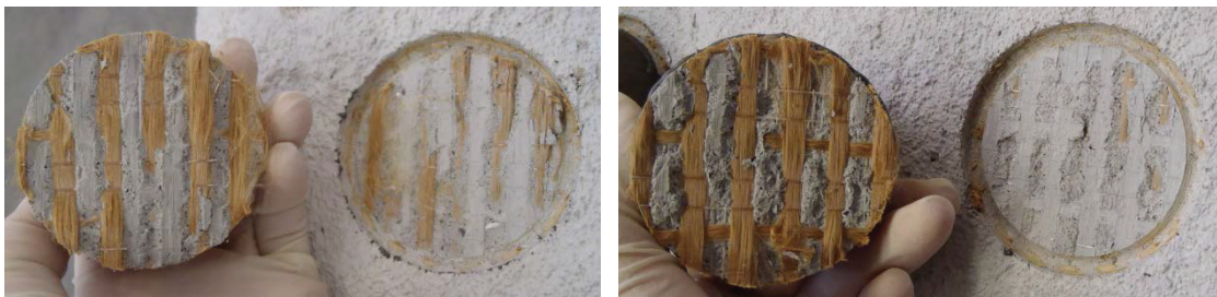
Figure 33 – Type “C” Failure Modes for 2 Plies (Left) and 4 Plies (Right)
