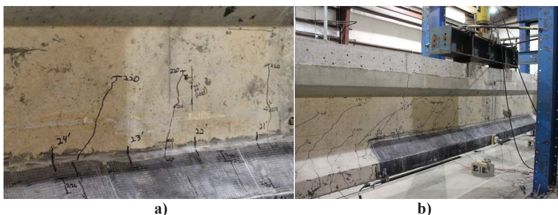
Figure 61 – Test C-3, Iteration 1 a) Crack Propagation b) Cracking Near Peak Load
