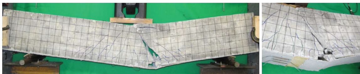
Figure 102 – Typical Fatigue Failure Mode for F-FRCM-1P-75 ( \beta^f=1.7\% )
