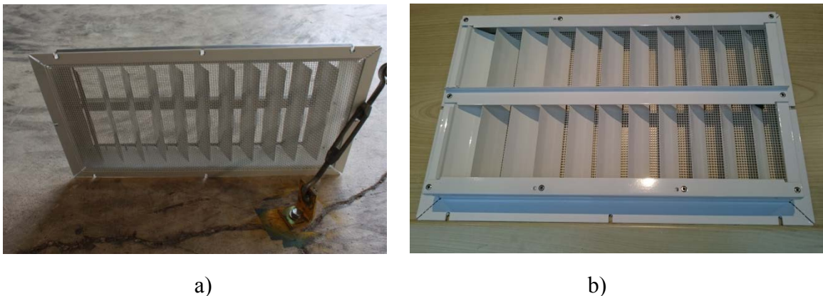
Figure 5-1. A valved soffit vent (VSV) that was used for this testing: (a) front; (b) back
