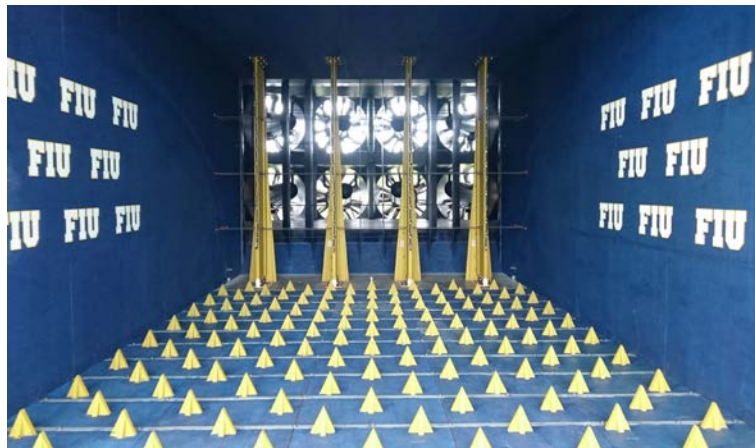
Figure 4-2. The WOW flow chamber with four spires and floor roughness elements
