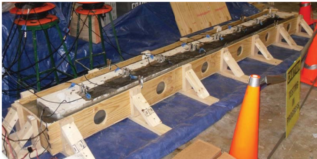
Figure 4.7 - Corrosion conditioning setup
