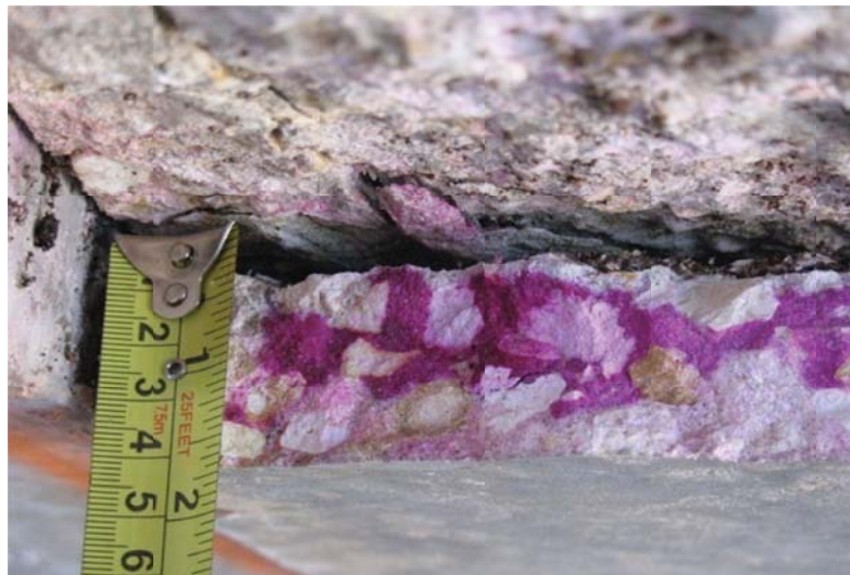
Figure 2.7 - Field exploration for carbonation detection
