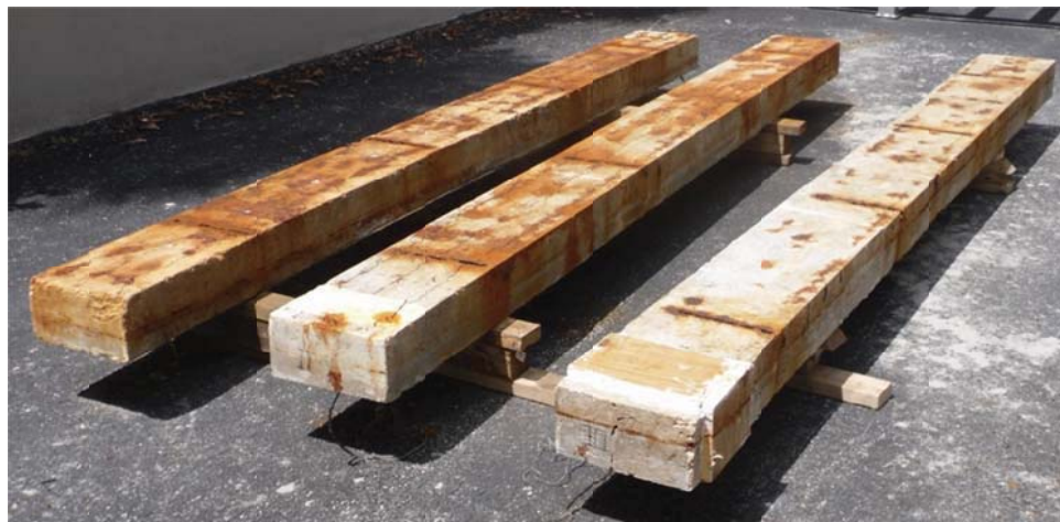
Figure 4.8 - Visual inspection after corrosion (B1 to B3)
