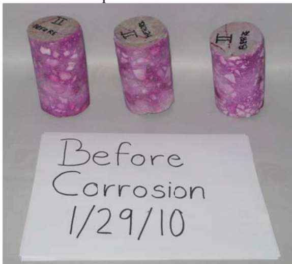
Figure III.D.2 - Core evaluation of concrete carbonation before corrosion
