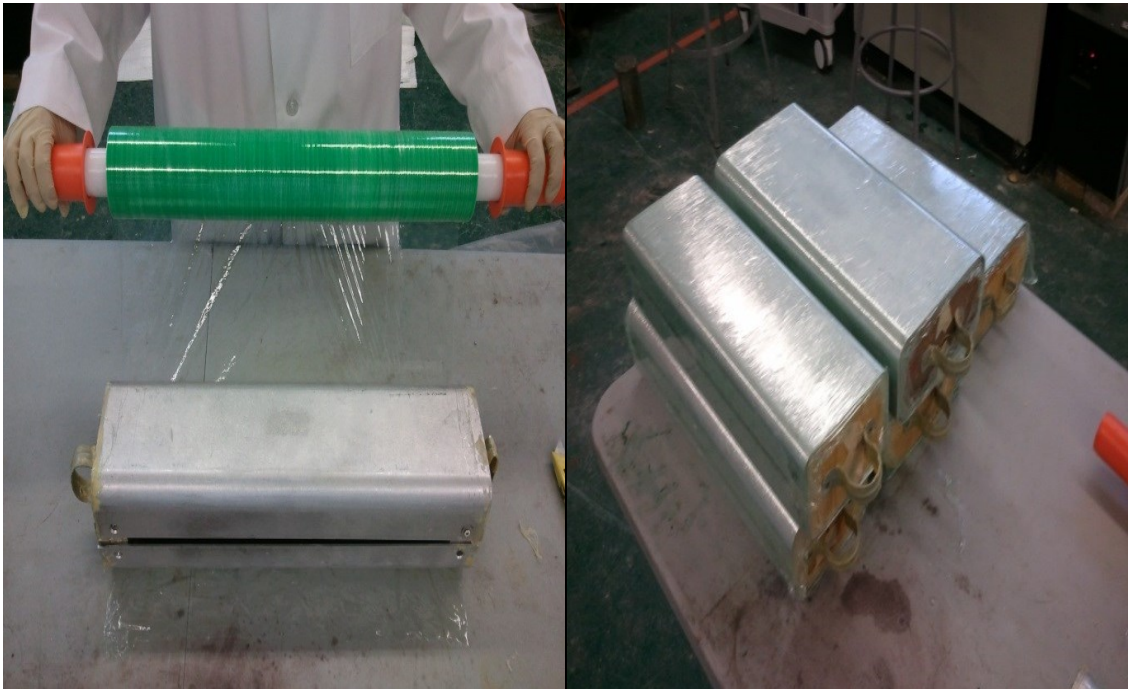
Fig. C-3: Aluminum "C" sections prepared for wrapping
