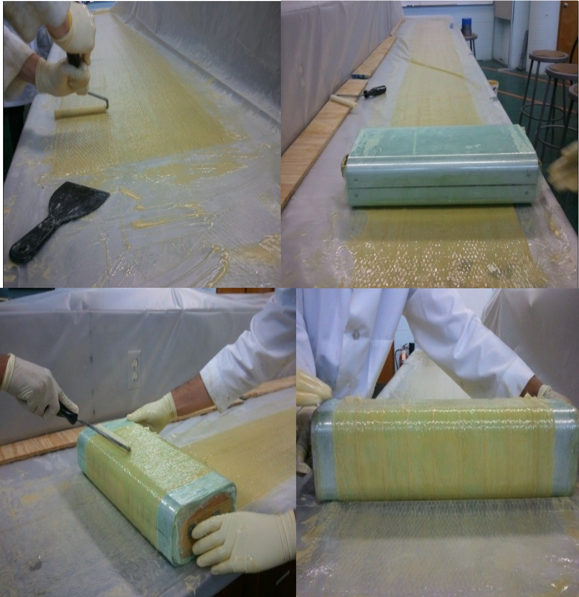
Fig. C-4: Wet lay-up impregnation of glass fibers and wrapping of the aluminum “C” section
