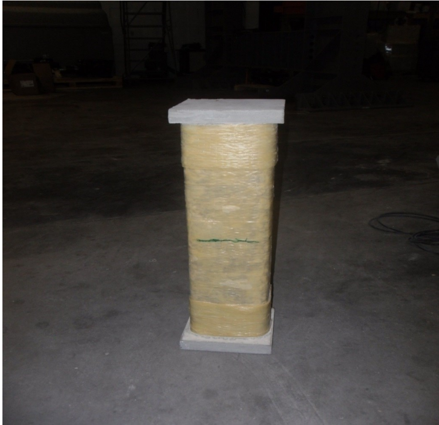
Fig. 3-2: Sample GFRP wrapped column
