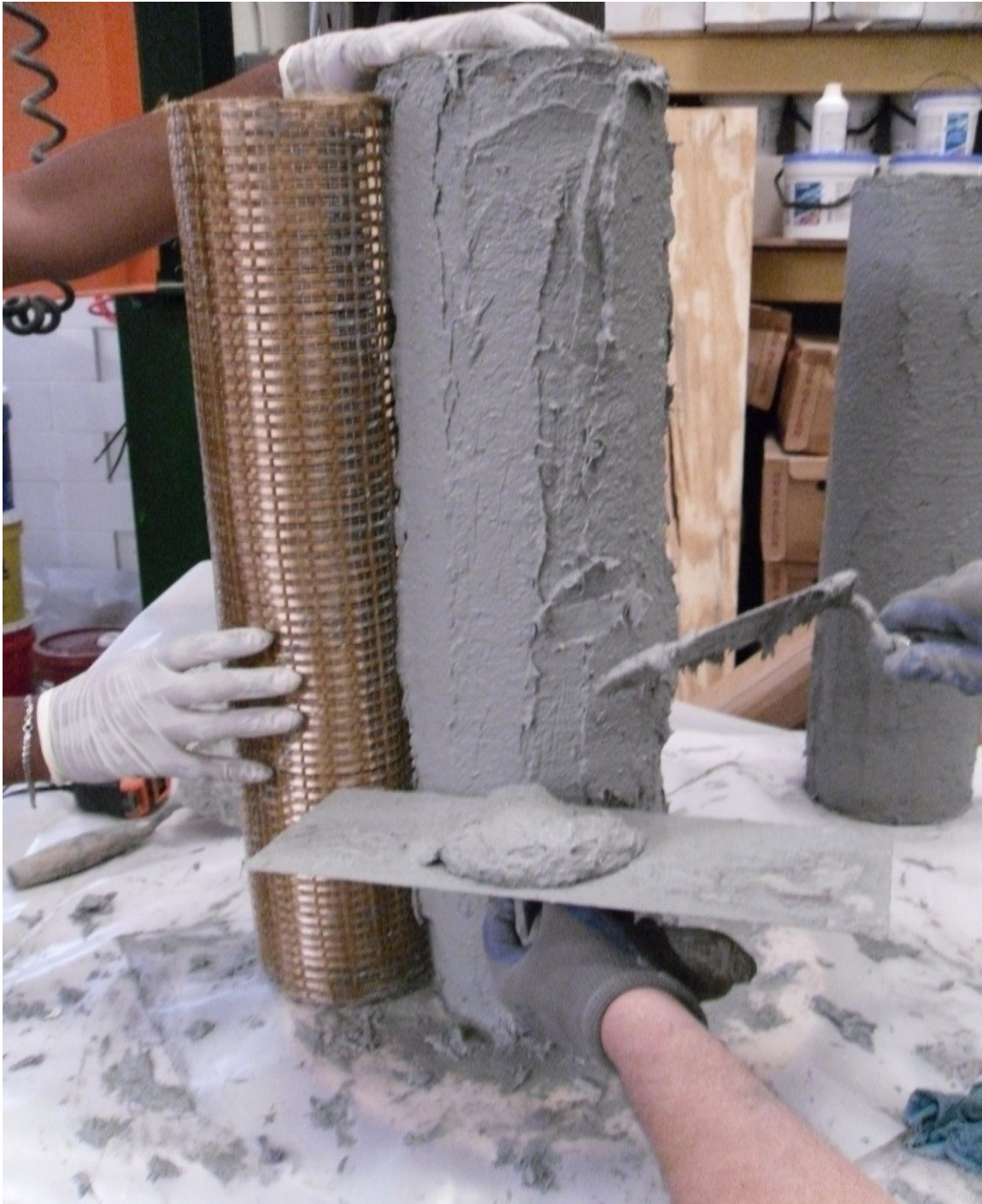
Fig. B-7: Application of the PBO fiber
