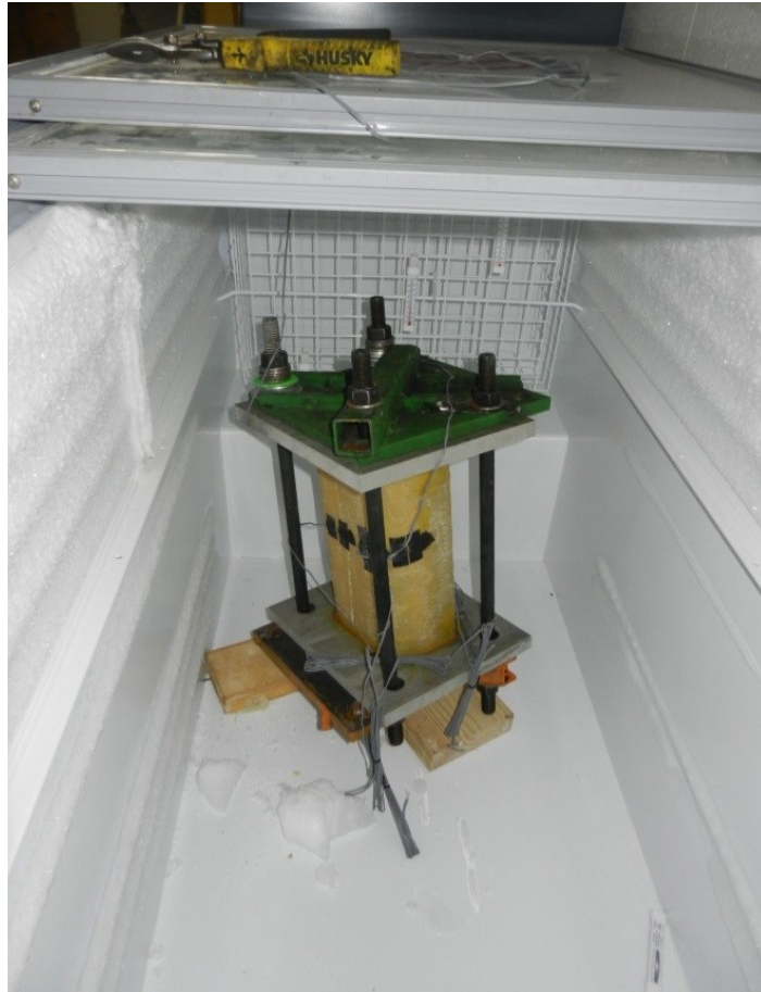
Fig. 2-4: Instrumented GFRP jacket inside the freezer
