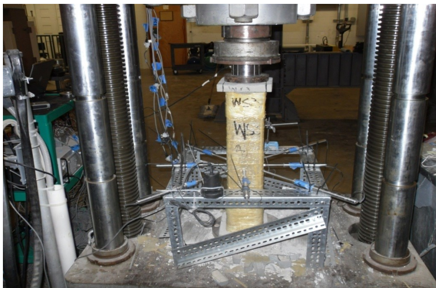
Fig. 3-3: Sample instrumentation and test set up
