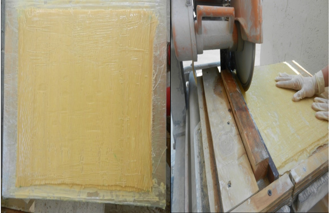
Fig. C-14: Curing of GFRP flat coupons and cutting the flat coupons in to standard sizes
