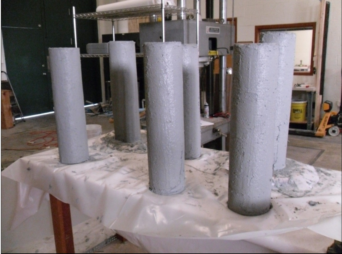
Fig. B-8: PBO-FRCM wrapped RC columns
