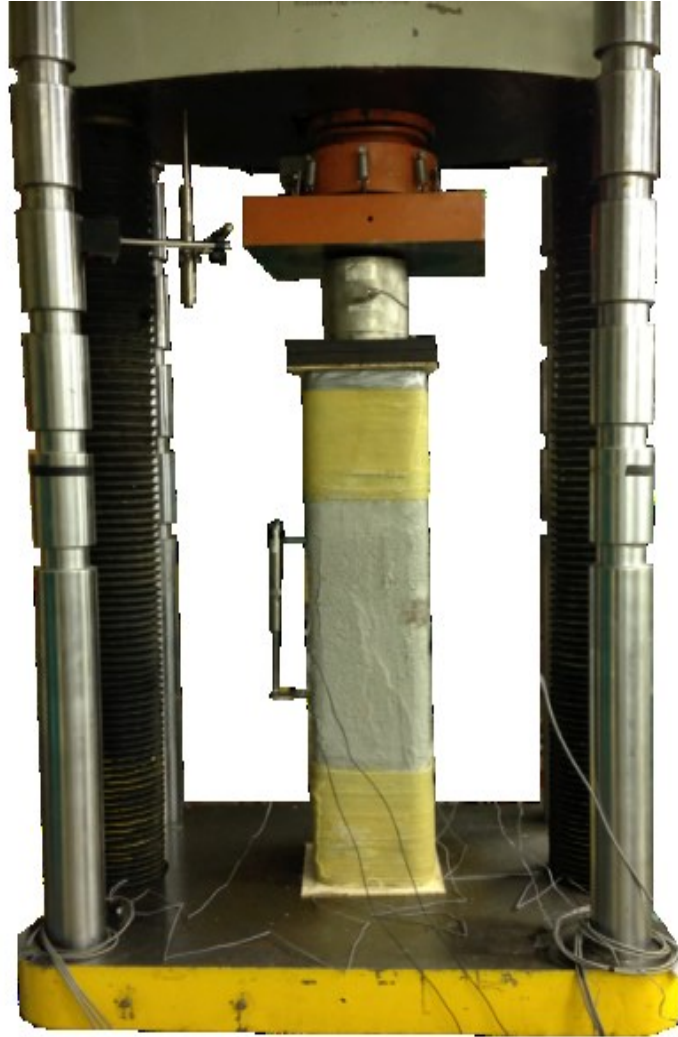
Fig. 4-3: Typical RC column specimen (square cross-section) before testing
