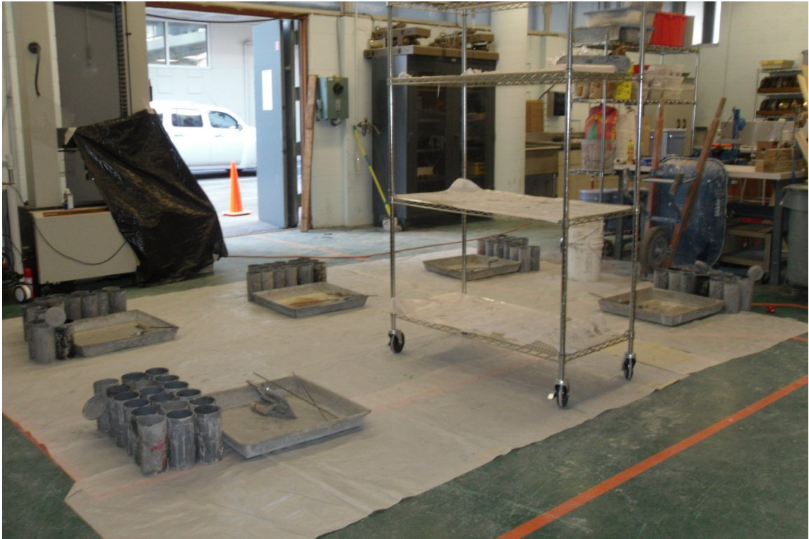
Figure B-1 - Setup for concrete mixing
