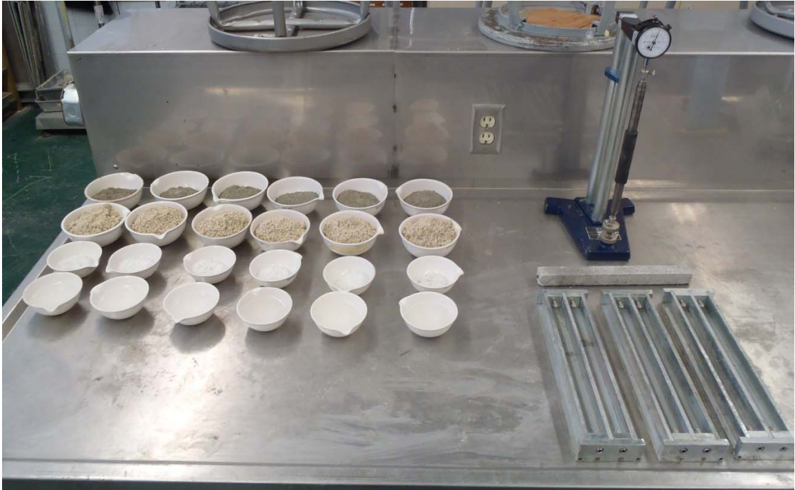
Figure A-1 - Setup for mixing ASR specimens
