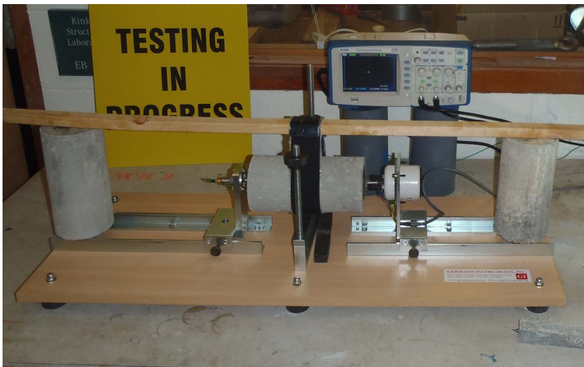
Figure B-12 - Fundamental longitudinal resonant frequency testing
