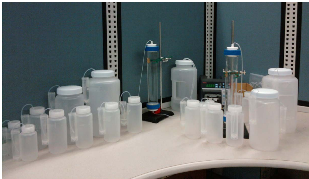
Figure A-8 - EPA Draft Method 1314 Percolation column setup
