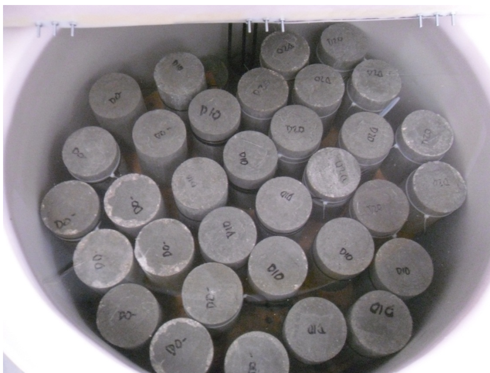
Figure B-7 - Arrhenius Aging setup
