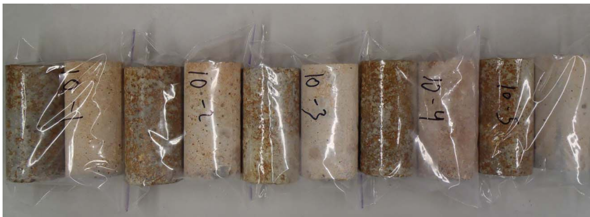
Figure C-30 - Discoloration from Diffusion samples. Lighter samples were exposed to the hot environment
