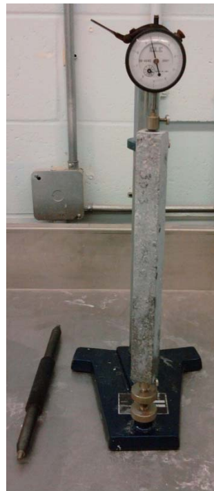
Figure A-3 - ASR specimen being measured
