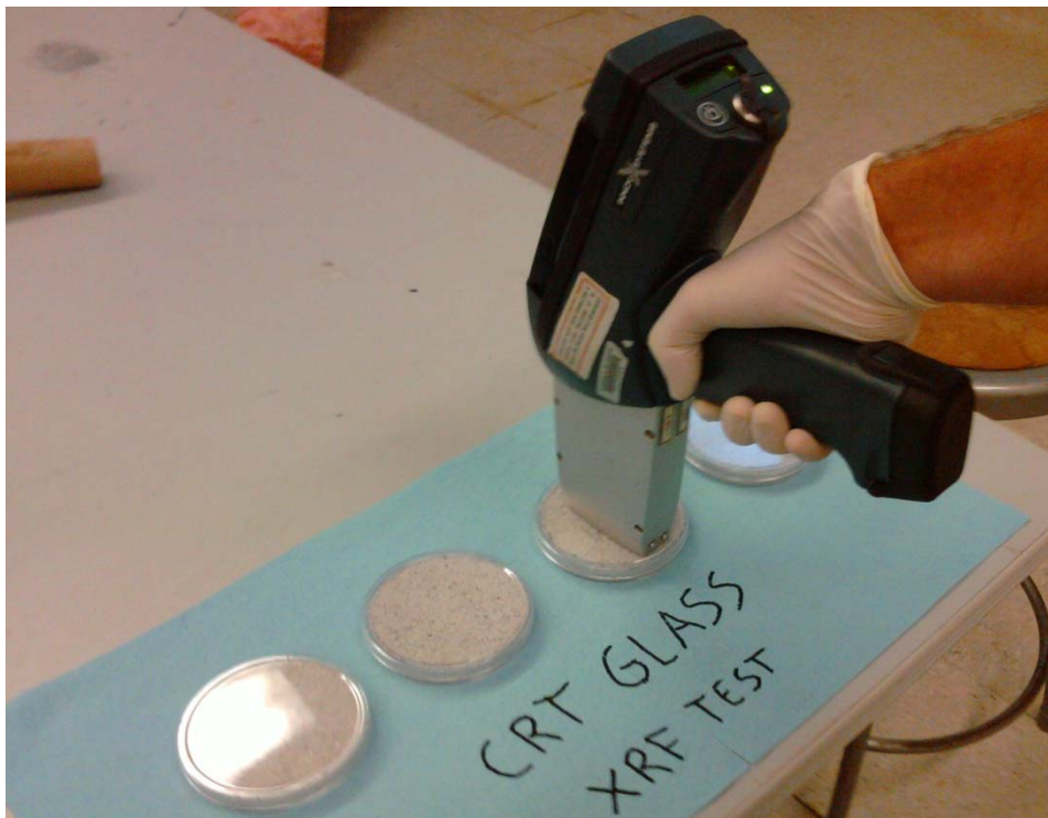
Figure C-1 - XRF testing of CRT glass
