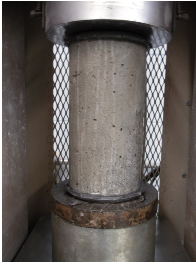
Figure A-5 - Compressive Strength Test
