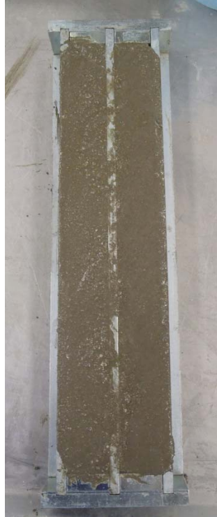
Figure A-2 - Fresh ASR Specimen in Mold
