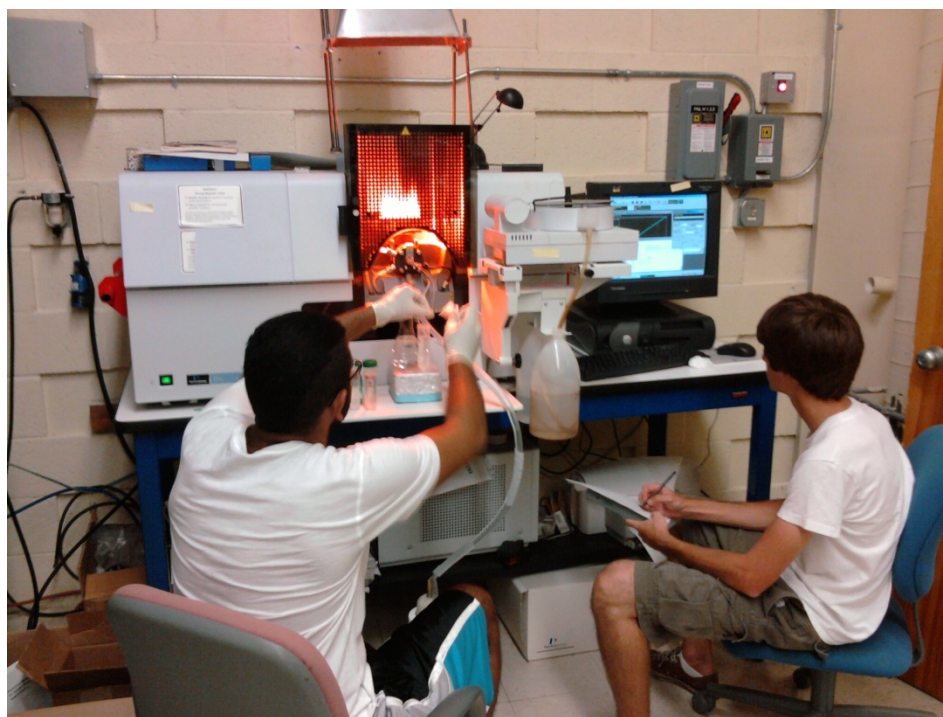
Figure A-7 - Atomic Absorption Spectrometer for constituent detection
