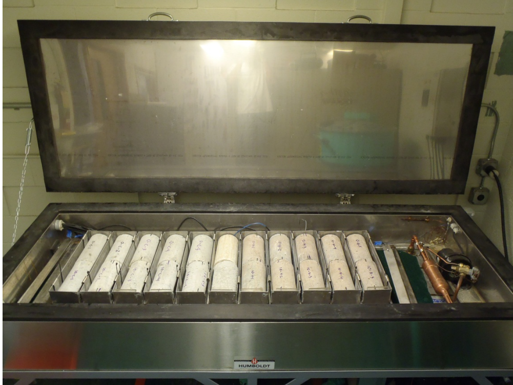
Figure B-8 - Freeze / Thaw testing setup
