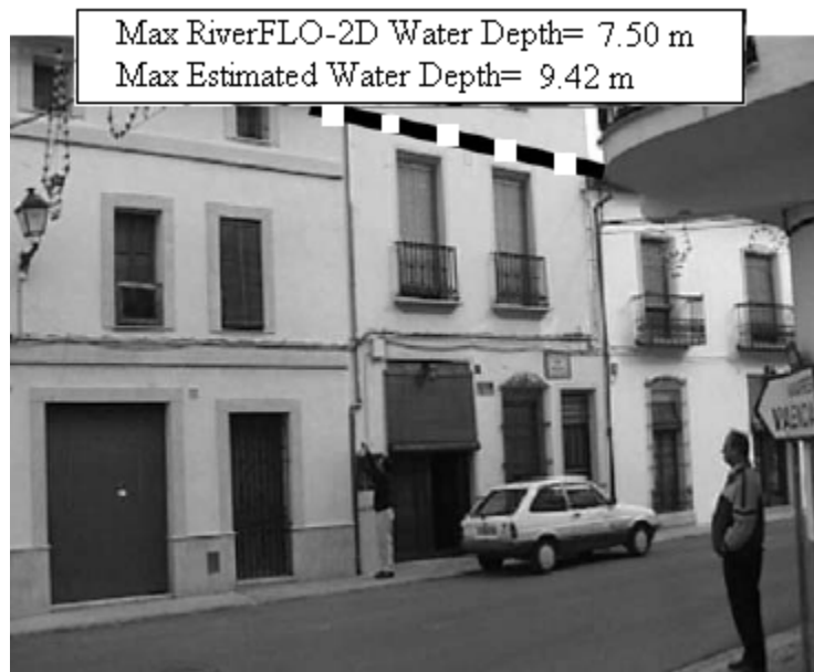
Figure 91. Sumacarcel Flooding Test. Water elevation mark and numerical water surface depth for gauge 3 in the Church Street of Sumacarcel.
