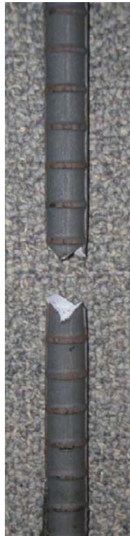
Figure 40 – Tensile Test on rebar
