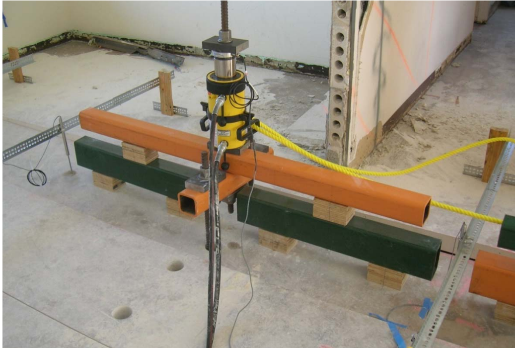
Figure 50 – Loading and Measuring Equipment
