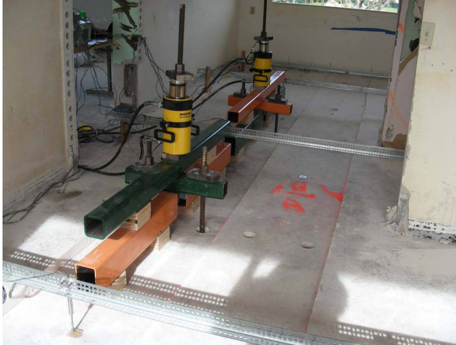
Figure 52 – Loading Setup (Hydraulic Jacks)
