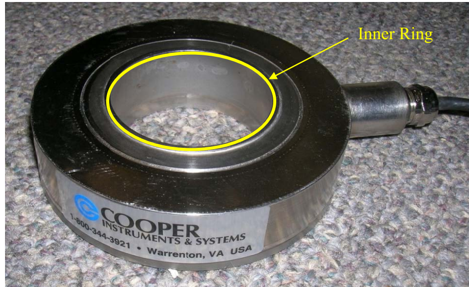
Figure 85 - Load Cell Loading Surface: Inner Ring
