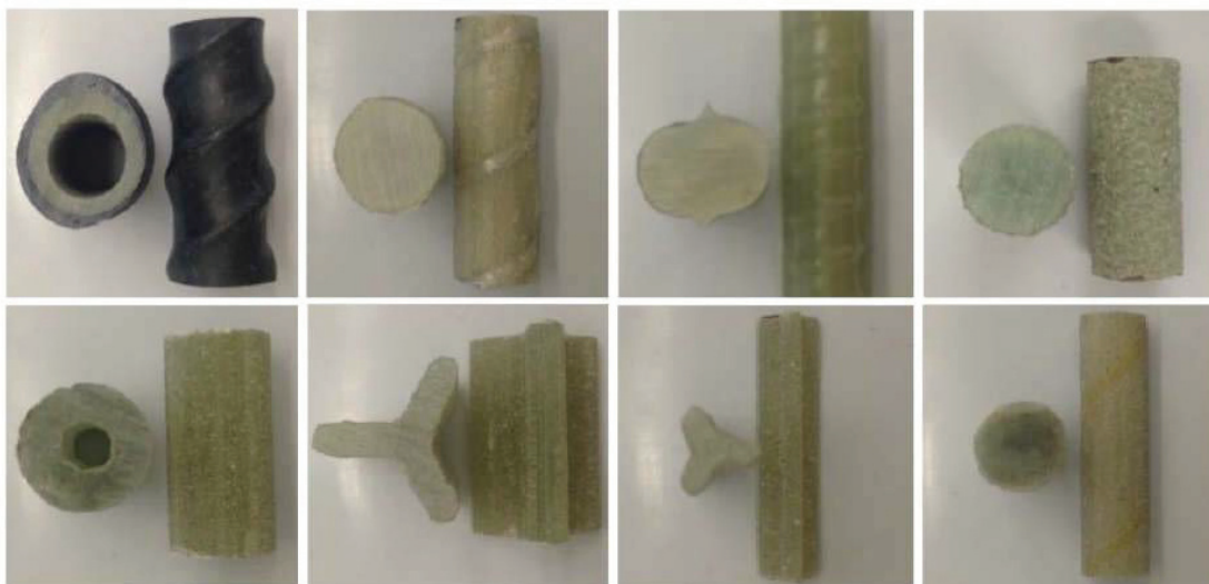
Figure 4 - GFRP rebar with different cross-sectional shapes [9]
