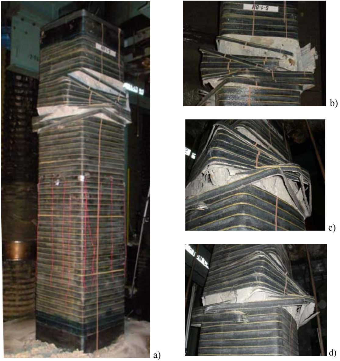
Fig. A - 25: Failure of Specimen S-1-8H (a-d).
