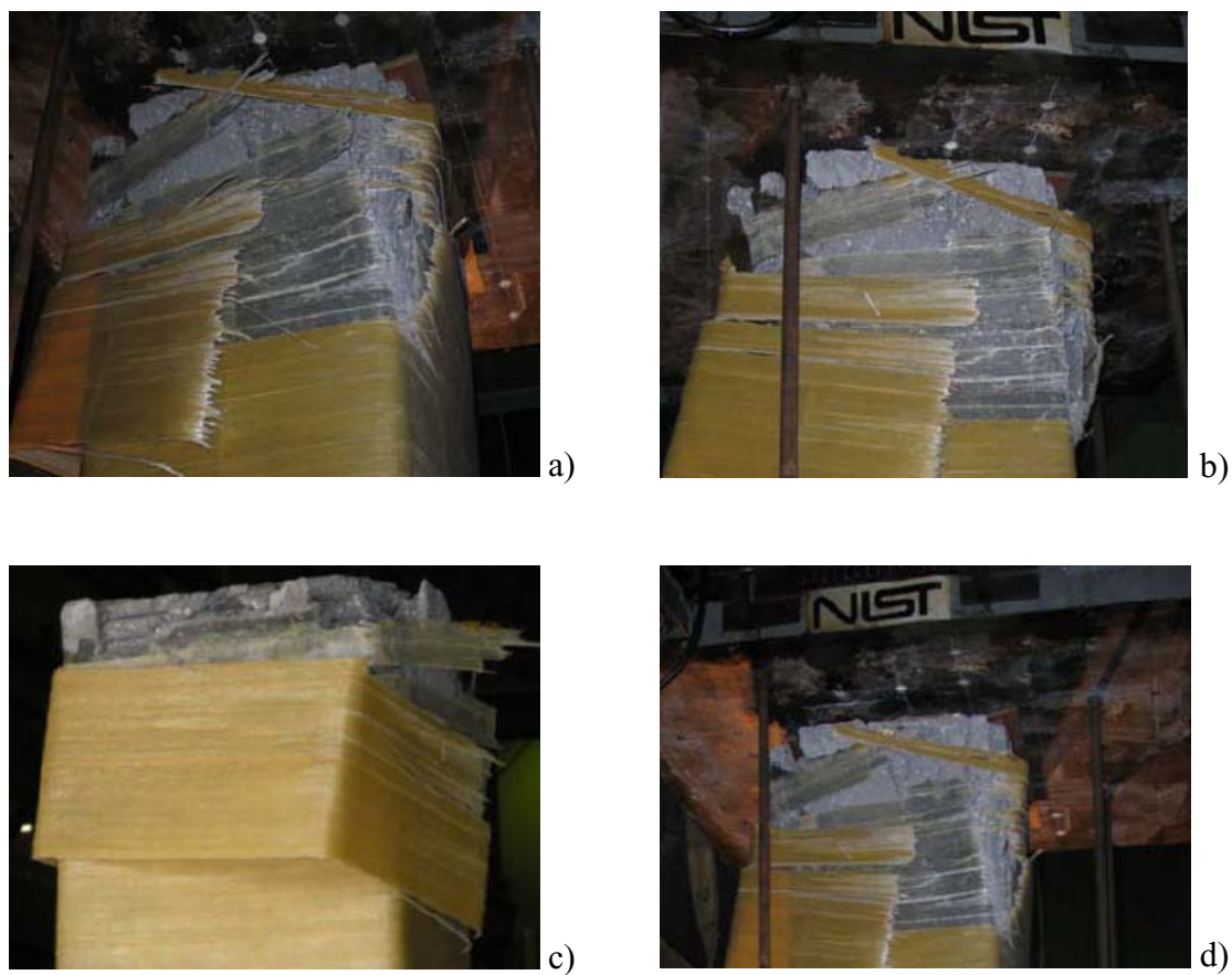
Fig. A - 27: Failure of Specimen R-1-5GA (a-d).
