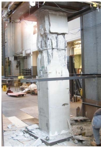
Fig. 3: Specimen S-16: normalized axial stress-normalized axial deformation response where the thick line shows the envelope curve (a); photograph of failed specimen (b); close-up of buckled steel bars (c).
