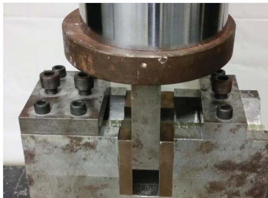
Figure 4.8: GFRP bars tested in transverse shear fixture
