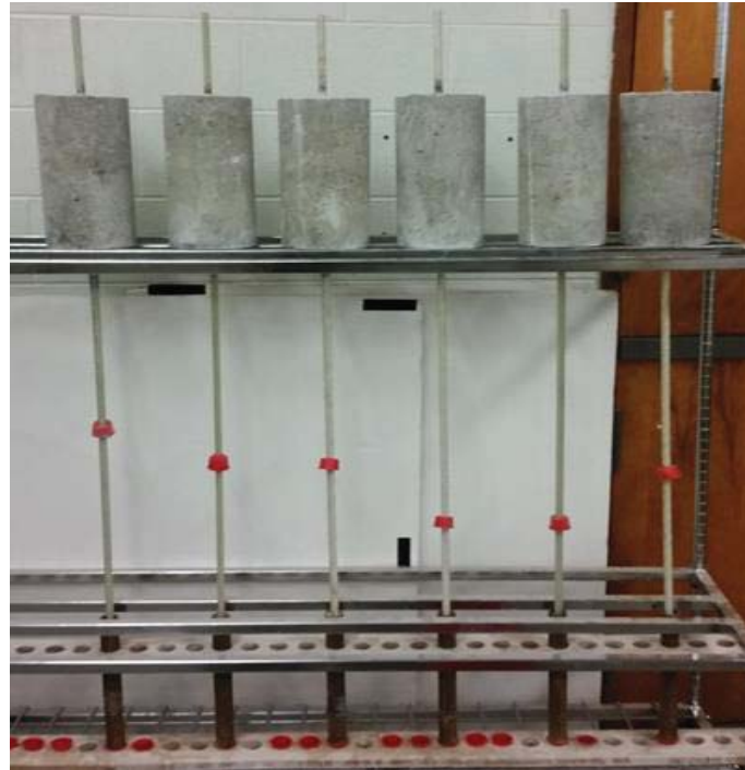
Figure 2.2: A set of prepared samples for the pull-out test
