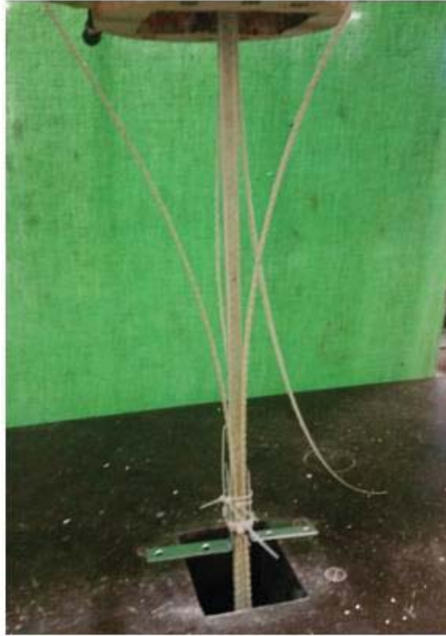
Figure 2.6: Failure of GFRP-C samples due to separation of surface enhancement layer
