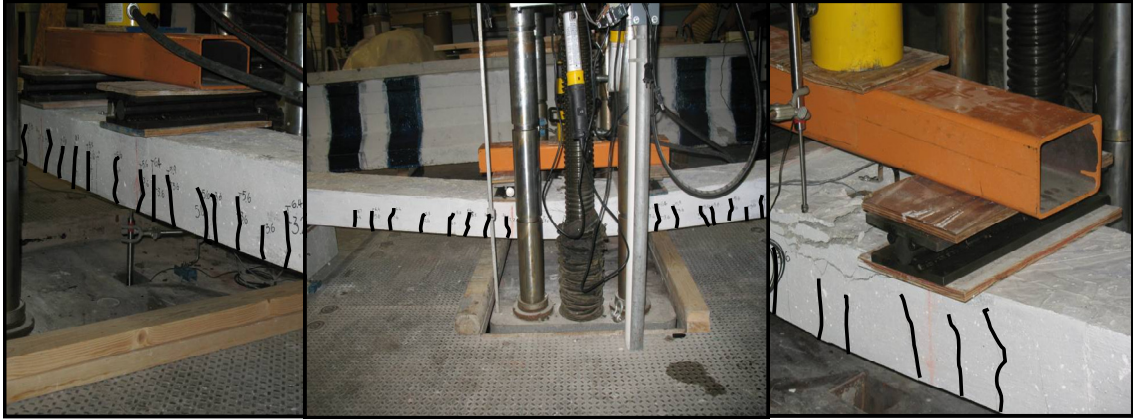
Figure 4.1 – Crack pattern and failure: control specimen
