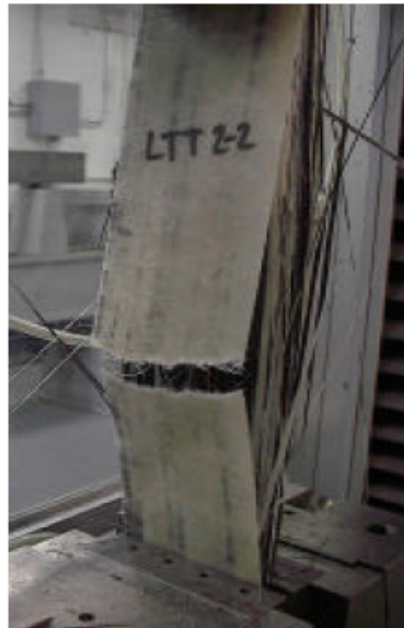
Figure 2.3 – Typical failure under tensile test in longitudinal direction (Arora, 2002)
