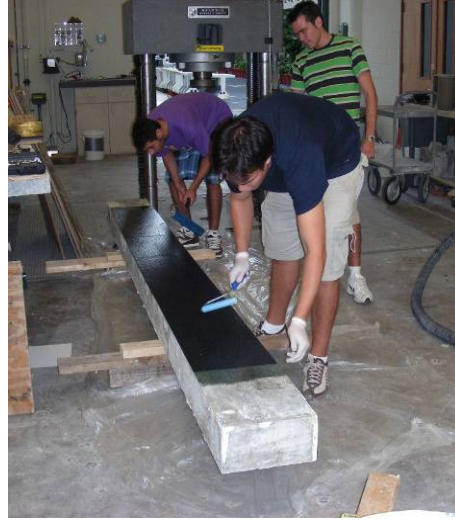
Figure 3.8 – Strengthening procedure of specimen EB
