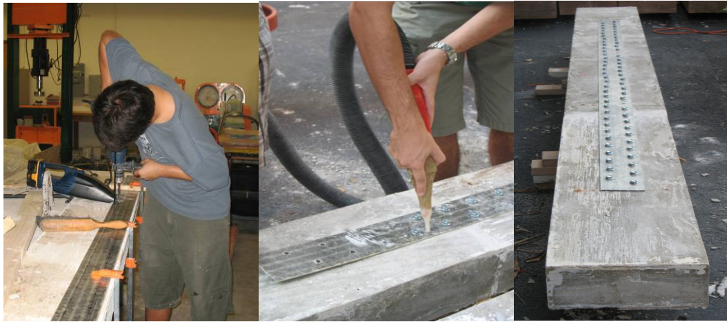
Figure 3.7 – Strengthening procedure of specimen MF-1-L
