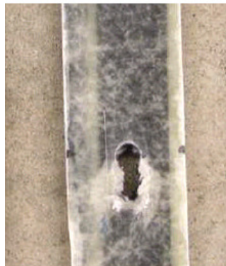
Figure 2.5 – Typical bearing failure observed (Arora, 2003)
