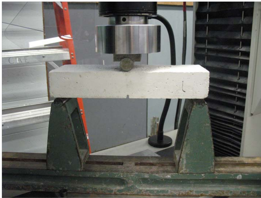
Fig. A.4 - 1– Three point bending set-up for sample cracking
