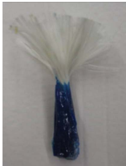
Figure 5.9 – Finished GFRP Spike
