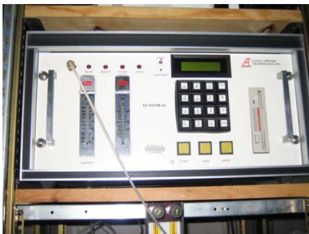
Figure 3.9 SF 6 collection and analysis system
