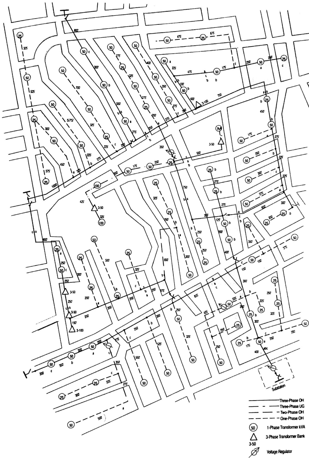
Figure 4.2: Electrical network overlaid on a map
