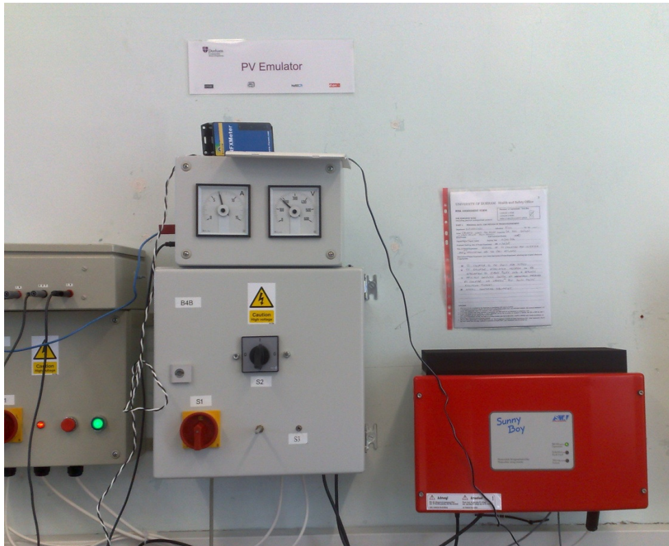
Figure 4.6: PV generation emulator at Durham University
