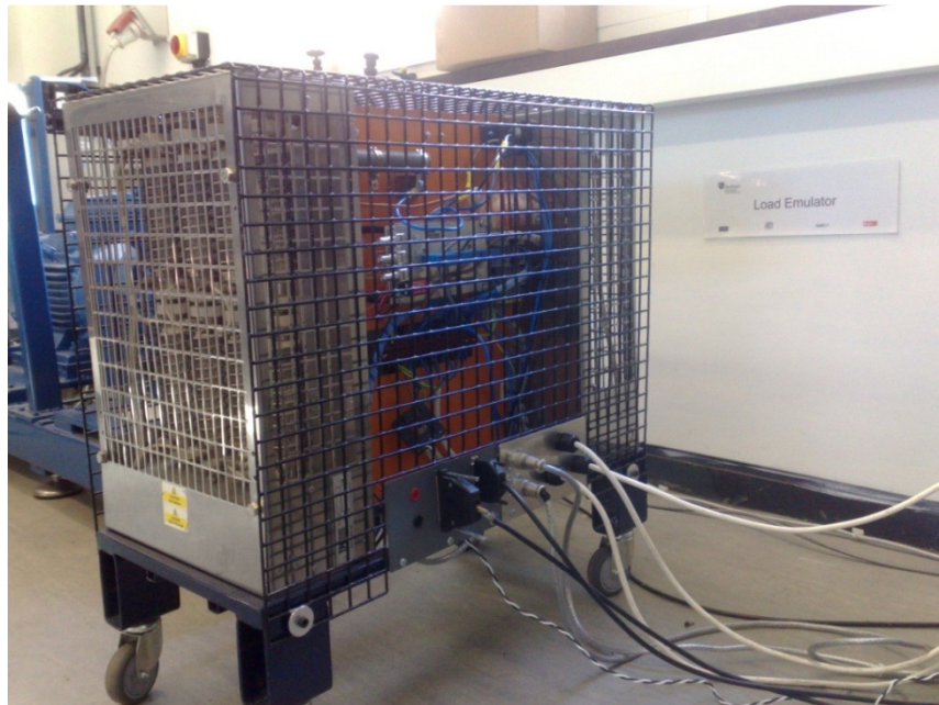
Figure 4.10: Load emulator at Durham University
