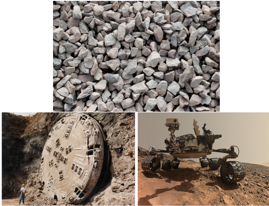
Figure 2.1: Photographs of granulate examples. Soil granulates can be found in nature in many shapes. Top: Gravel aggregate frequently used in construction. Left: A Tunnel boring machinery shield. Rock jamming can occur during phases of drilling, crushing, extraction. Right: Movement of rover Curiosity on Martian soil granulates. Non-spherical particle interaction (rolling resistance, particle displacement, bulldozing effect) with rover wheels is an important research area in the field of terra-mechanics and robotics where soil samples are not widely available for laboratory experiments. 1
