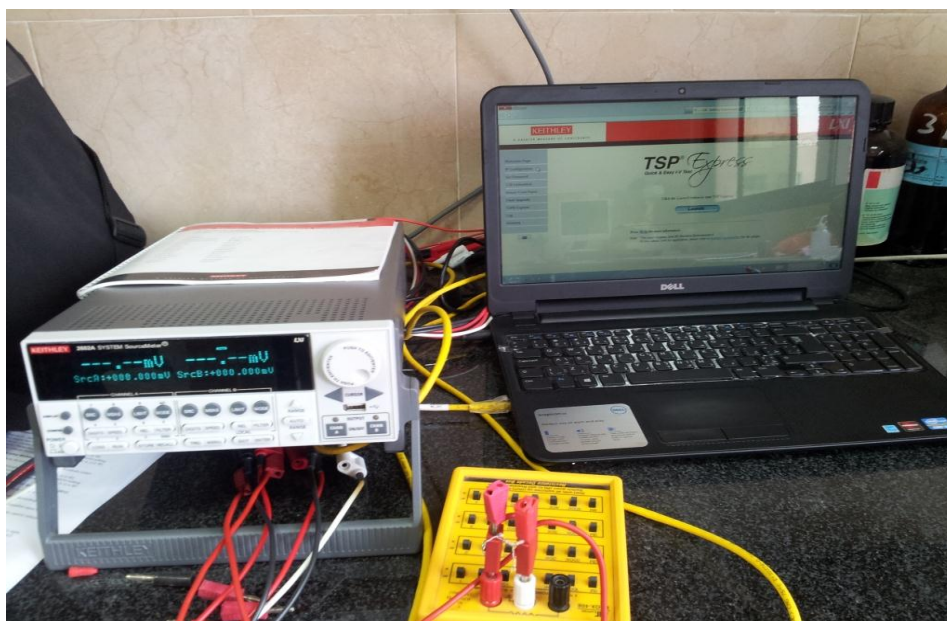
Fig. 3. 6. Photo image of J-Vmeasuring setup.
