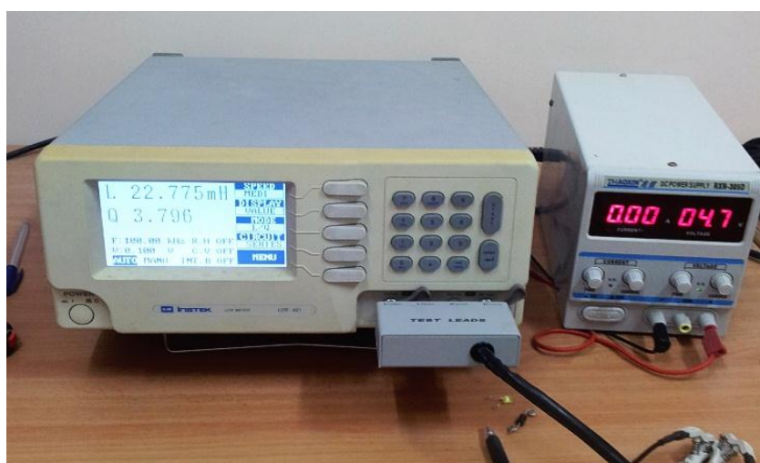
Fig. 3. 8. LCR-821 instrument that is used in C-V measurements.
