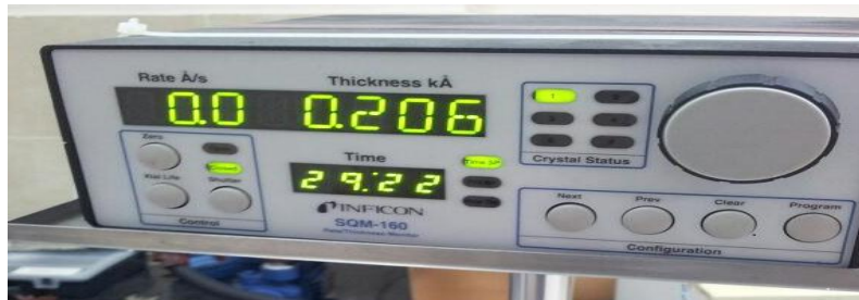
Fig. 3. 5. A SQM-160 quartz crystal monitor that used to know the thickness of film deposition.
