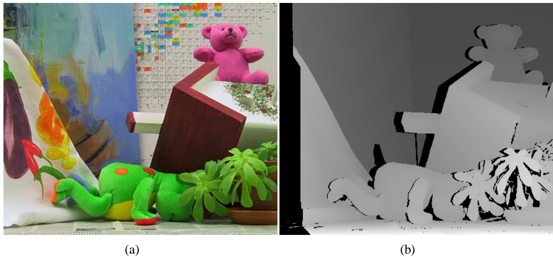
Figure 5.4: Shows how the intensities of the occluded area are available in the stereo image: (a) the original stereo image (b) Its disparity with occluded area masked in black.
