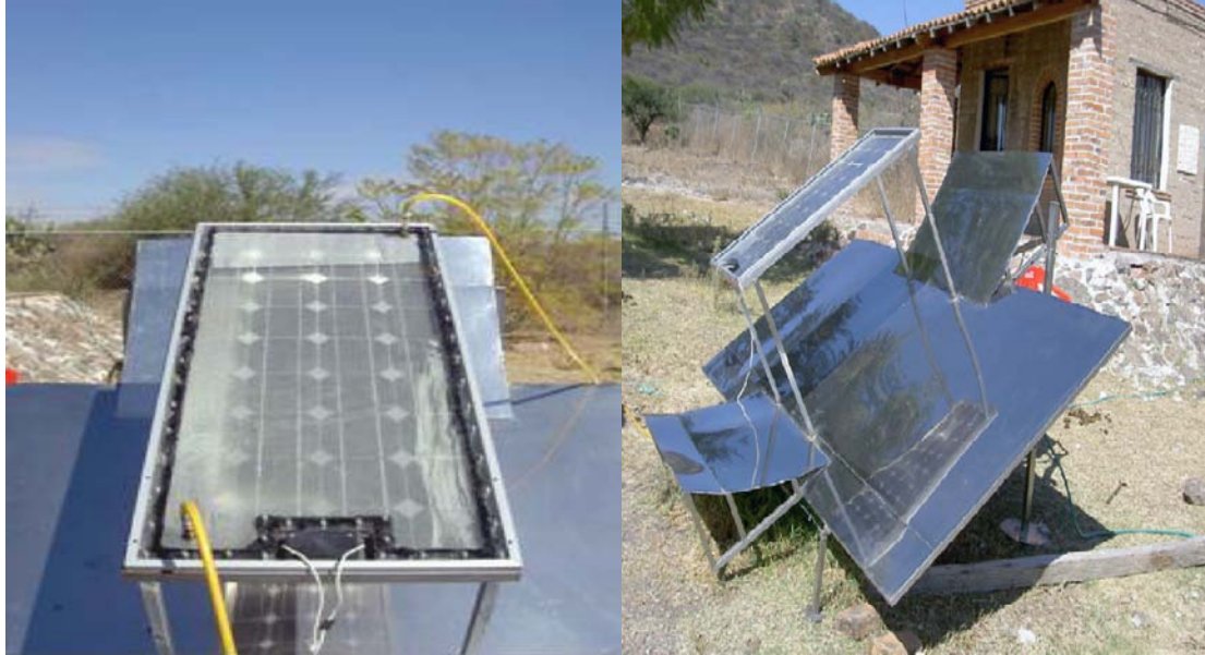
Figure 2.9k A bifacial PV module [69].
