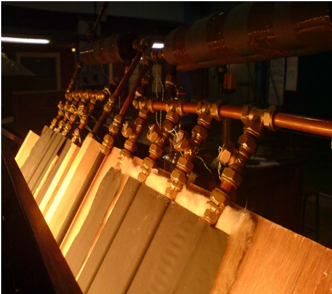
Figure 6.3b Collector with thermocouples attached and insulated water jackets.
