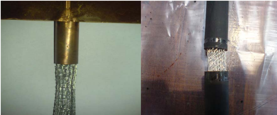
Figure 6.2e Porous medium inserted in a copper pipe.
