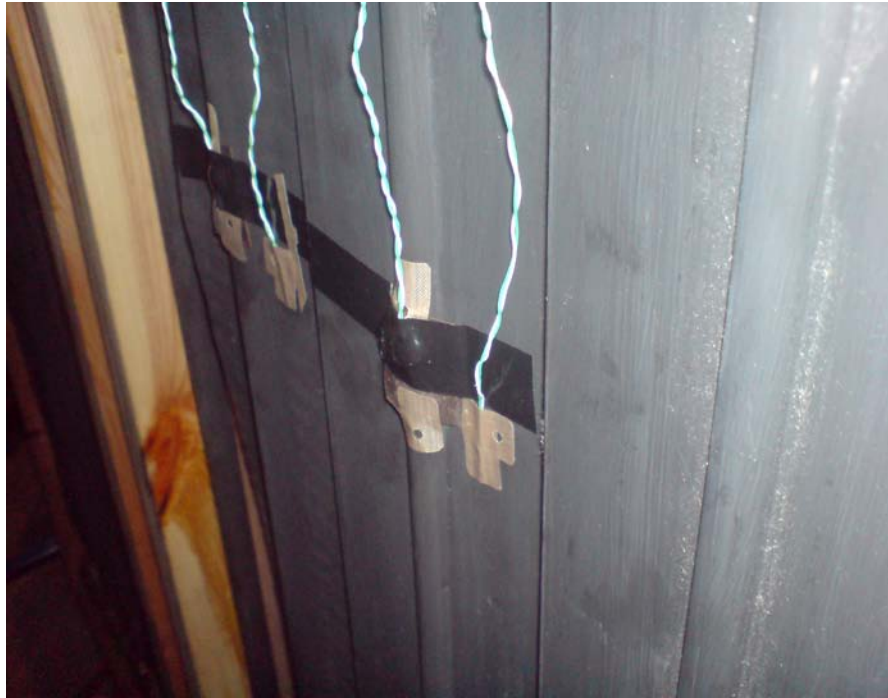
Figure 6.4j Surface temperature measurements setup.
