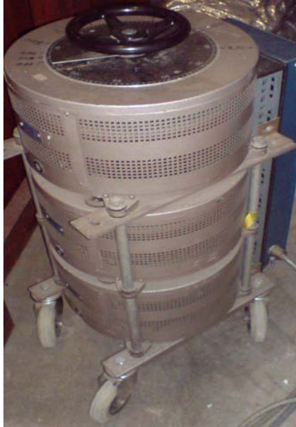
Figure 6.2d A three phase electrical transformer.
