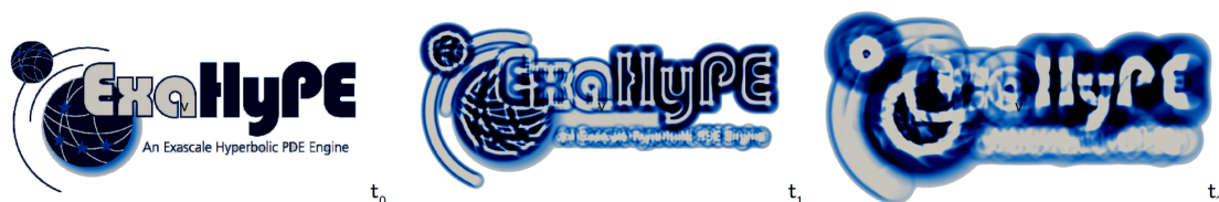
Figure 1.1: A simple visualisation of the 2D Euler equations with the logo of the ExaHyPE project as initial conditions.
