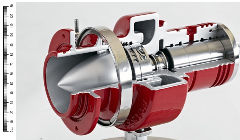
Figure 4.1: Cut-Through Cummins Waste Heat Turbo Expander Unit [27].
