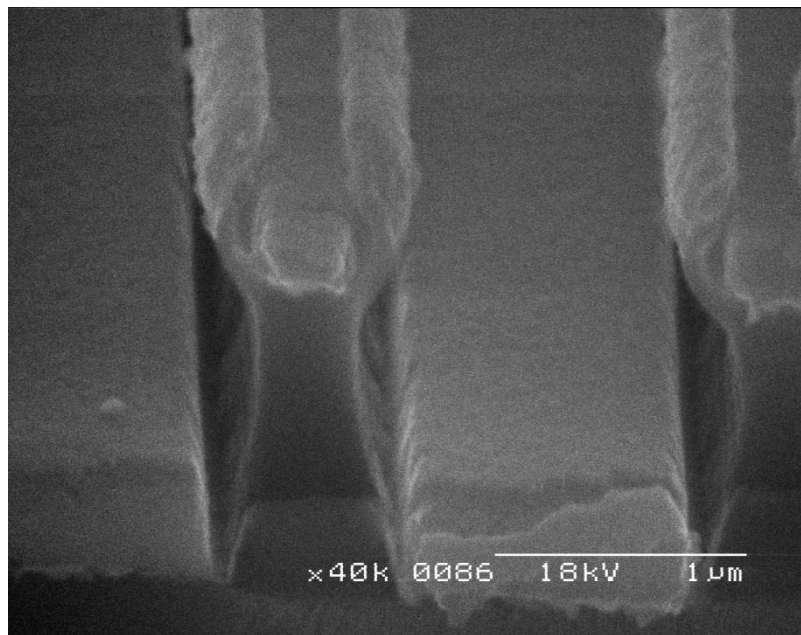
Figure 3.6 – An SEM showing a 500 nm layer of Ni (e-beam deposited over a line feature formed using the single-layer lift-off process) which caused curling of the photoresist
