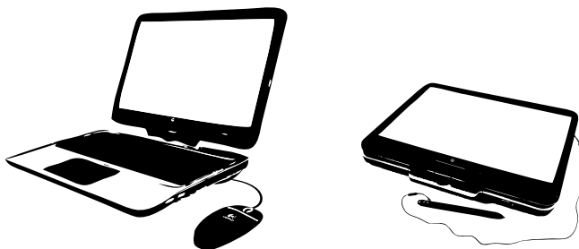
Figure 7. HP TouchSmart tm2 in “laptop mode” with mouse ( left ) and in “tablet mode” with stylus ( right ).
