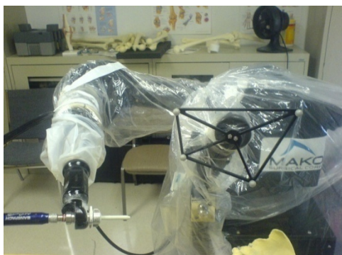
Figure 2.16: MAKO Surgical Corp.'s approach with a camera tracking a tibia, femur, and robot. a) A phantom tibia with a 4-sphere tracker pinned to the bone. b) A phantom femur with a 4-sphere tracker pinned to the bone. c) The robot manipulator arm with cutting device attached and 4-sphere tracker fixed to the base. d) Infrared camera (Northern Digital Imaging Inc., Waterloo, Canada) that has a view of all three trackers. Infrared LED's can be seen emitting light from the camera "eyes".
