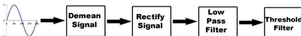
Figure 4.9: Bone intra-signal processing flowchart. A sinusoid is shown as a sample input signal to the series of filters that ultimately find a peak from a bone reflection. The demean filter finds the average value and removes it from each element in the signal. Rectify signal takes the absolute value of the signal so the successive filters will only perform operations on non-negative values. The low-pass filter smoothes out the signal so contiguous peaks and valleys can be easily detected. The threshold filter analyzes the smoothed result and determines how many significant peaks exist.
