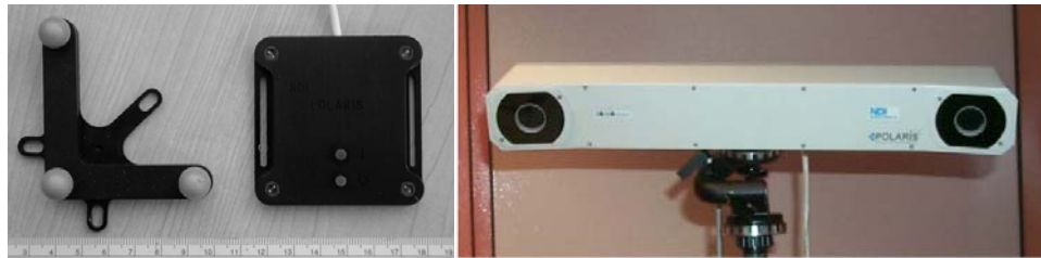
Figure 2.7: Trackers and stereoscopic cameras work together to determine physical three-dimensional information [77, 81]. On the left, passive and active trackers are used in a study to determine the accuracy of optical tracking. These trackers are attached to the bone using stereotactic frames or bone pins and clamps. The left tracker is passive and has reflective spheres attached to the frame. The right tracker is active and has LED's embedded in the frame to generate a signal rather than reflect one. On the right, a stereoscopic camera (Northern Digital Imaging Inc., Waterloo, Canada) has two sensors that detect trackers and triangulate their position in three dimensions. Infrared beam emitters are located on the face of the camera for use with passive reflecting trackers.
