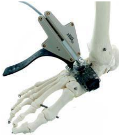
Figure 2.13: Optically tracked device for capturing ankle center [66]. Instead of capturing the medial and lateral malleoli and calculating the ankle center from that, this device can more accurately determine the ankle center based on kinematic motion of the ankle joint. This leads to a more accurate rough registration which provides a better initial guess for the registration routine.
