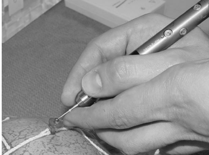
Figure 2.5: An Acustar fiducial cap is used for a fiducial-based registration [52]. The user is holding an optically tracked instrument that is precisely indicating the position of the fiducial marker. Several fiducial markers can be used to create an accurate registration between an image space model with radiopaque markers and a physical model with the embedded markers accessible to a pointer.
