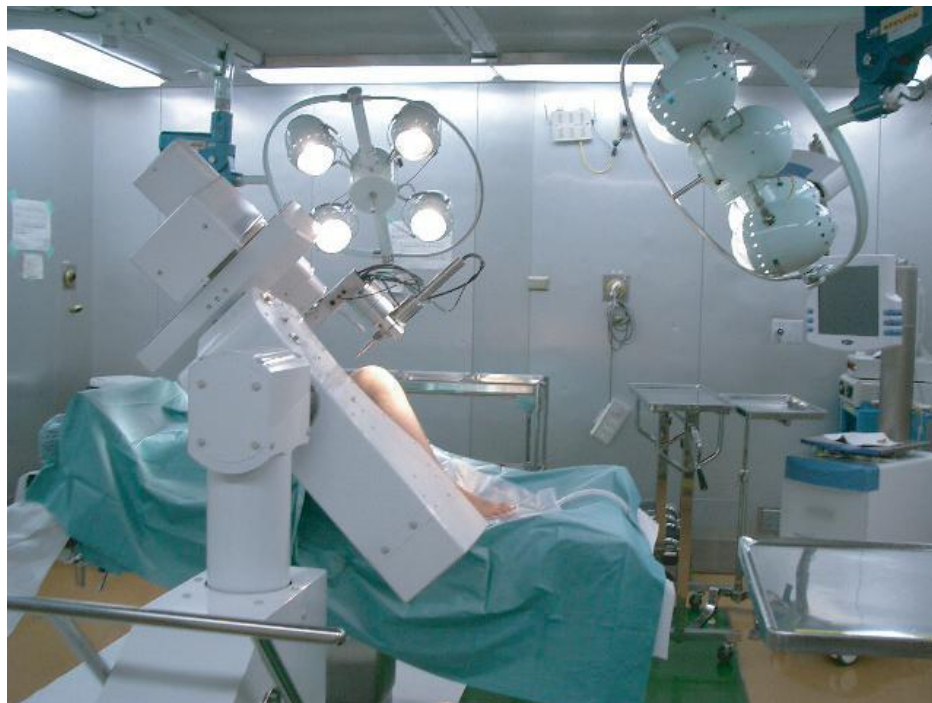
Figure 2.12: Seven degree-of-freedom robot using a preoperative plan and registration to perform Unicondylar Knee Arthroplasty (UKA) [68]. The robot is shown poised over a patient's knee. The registration and navigation components are provided by a BrainLAB VectorVision system. The robot uses an optical tracking system to locate the pointer for registration.
