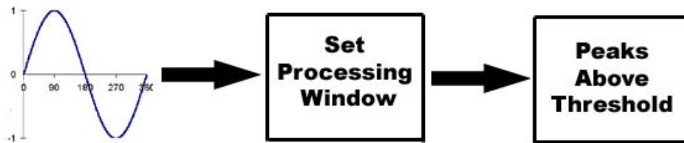
Figure 4.5: Processing scheme for calibration signals. The sinusoid shows a sample input that is passed through two filters. A processing window establishes a minimum and maximum distance in between which the peak is expected. If the peak occurs outside this window, it will not be detected. This implies that the transducer should be held an appropriate distance from the surface of the phantom. The signal is then passed through a peak detection filter that looks for intensities above a certain threshold.
