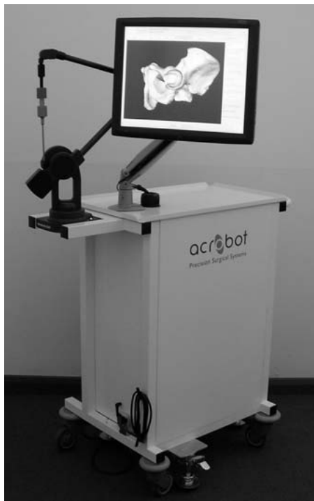
Figure 2.10: Acrobot navigation system incorporating a mechanical tracking arm and touchscreen display [6]. This system is used for hip replacement surgery. It employs a region-based surface-match registration.
