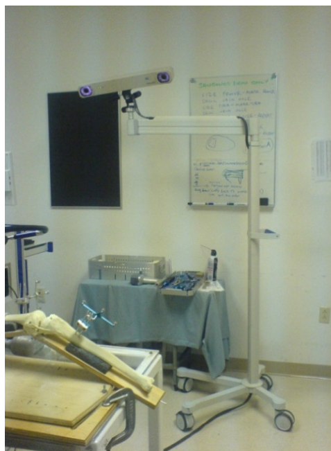
Figure 2.16: MAKO Surgical Corp.'s approach with a camera tracking a tibia, femur, and robot. a) A phantom tibia with a 4-sphere tracker pinned to the bone. b) A phantom femur with a 4-sphere tracker pinned to the bone. c) The robot manipulator arm with cutting device attached and 4-sphere tracker fixed to the base. d) Infrared camera (Northern Digital Imaging Inc., Waterloo, Canada) that has a view of all three trackers. Infrared LED's can be seen emitting light from the camera "eyes".
