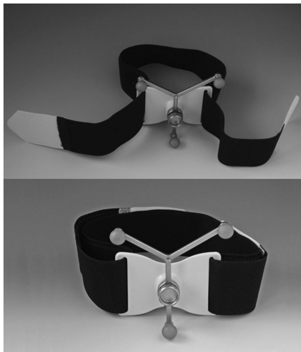
Figure 2.9: Headband with passive reflective markers for optical tracking [39]. The headband proved to be too mobile during the surgery to maintain a clinically accurate registration.
