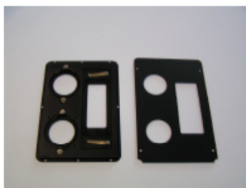
Figure 11: Interchangeable plate adapters for 2 well, glass slides and 96 multiwell
