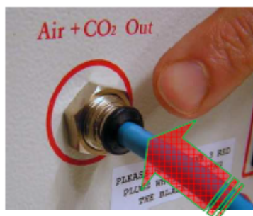
Figure 4: Avoid gas leak: strongly push the tube into the Swift-Fit connector
