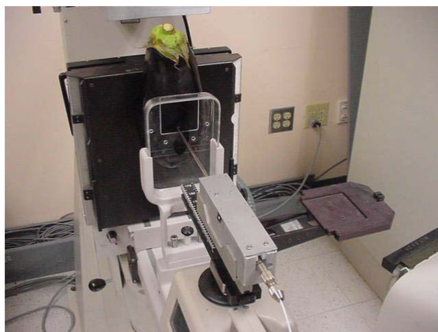
Figure 3.30 : The insertion of the optical fiber into an eggplant using the fiber-insertion system
