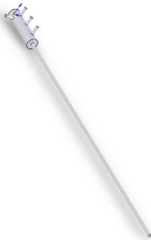
Figure 3.20: The trocar of the fiber-insertion system consists of an aluminum trocar needle, a Plexiglas trocar handle, and four steel dowel pins (Small Parts, Miami, FL). The two pins nearest the distal end of the trocar are locking pins. The two other pins are rotating pins. The rotating pins are used to unlock / lock the trocar and retract / insert the trocar (Hoang M 2006).
