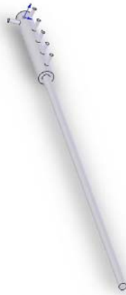
Figure 3.19: The cannula of the fiber-insertion system consists of an aluminum cannula tube, a Plexiglas cannula handle, and six stainless steel dowel pins: five locking pins in series along the length of the handle and one rotating pin located at the edge of the cannula handle and perpendicular to the locking pins. The inner diameter of the cannula tube was chosen to allow insertion of the fiber clamp in which the optical fiber will be inserted. The locking pins were spaced such that the cannula may be retracted at 1 cm increments (Hoang M 2006).
