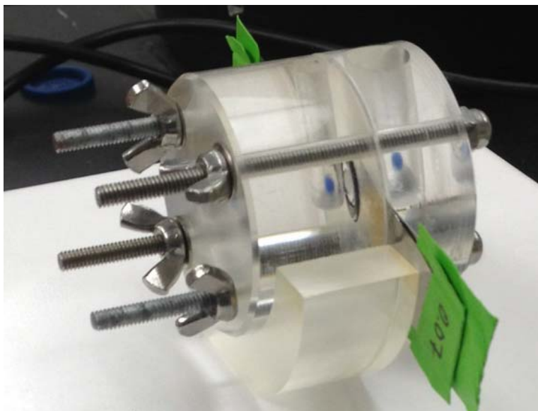
Figure 4-4 Photograph of the actual diffusion chamber used during an experiment on a magnetic stirring plate. The metal spacers were used to confine the specimen to its desired thickness and could be increased in order to compress the tissues to 10% or 20%, as needed.
