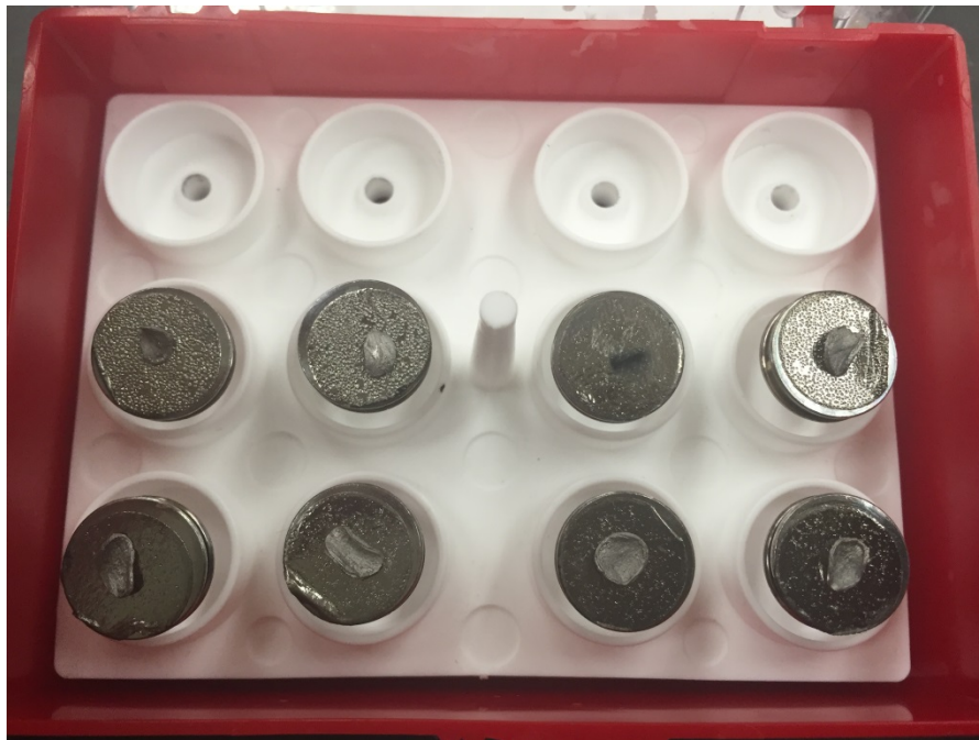
Figure 4-6 Photograph showing the knee meniscus tissue samples prepared for scanning electron microscopy. The samples were fixed with a 2% glutaraldehyde in PBS solution. Samples were then be dehydrated in a graded series of ethanol (20%, 50%, 70%, 90%, 100%) and dried by immersion in hexamethyldisilazane. Tissue specimens were taken in both the axial and circumferential direction in order to compare the collagen alignment.
