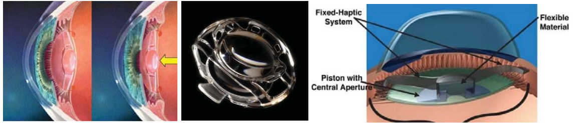
Figure 2.3: (Left) A single-optic IOL and a demonstration of its principle of operation ( www.marineyes.com ). (Middle) A dual-optic accommodating IOL, with both optics joined via the IOL's haptics (Bohorquez & Alarcon, 2010). (Right) A deformable IOL with components labeled. Note how the optic sits on the capsular bag (Alio et al, 2009).
