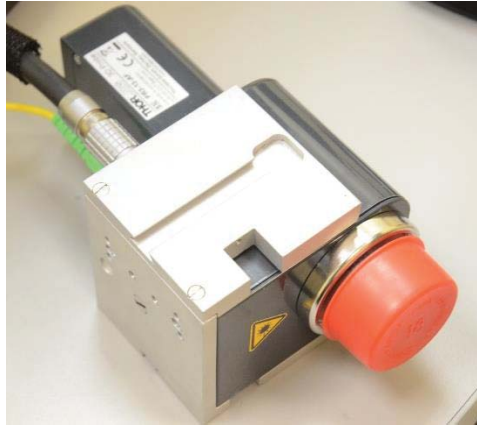
Figure 5.9: The trans-scleral SD-OCT probe affixed to the custom U-bracket with a female dovetail feature on either side to allow for mounting on either side of the main system base.
