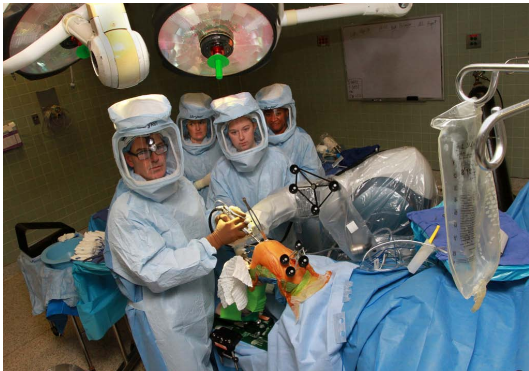
Figure 2-15: Photography of MAKO RIO system used in operating room (Copyright Gray Whitley. Picture retrieved June 19, 2011, from http://www.flickr.com/photos/gray_whitley/5439904479/ ).
