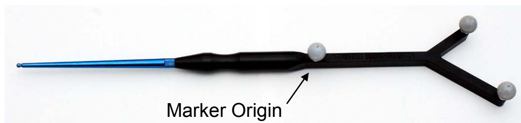
Figure 3-2: Picture of a mechanical probe. Three reflective spheres are attached in a unique pattern and form an optical marker.
