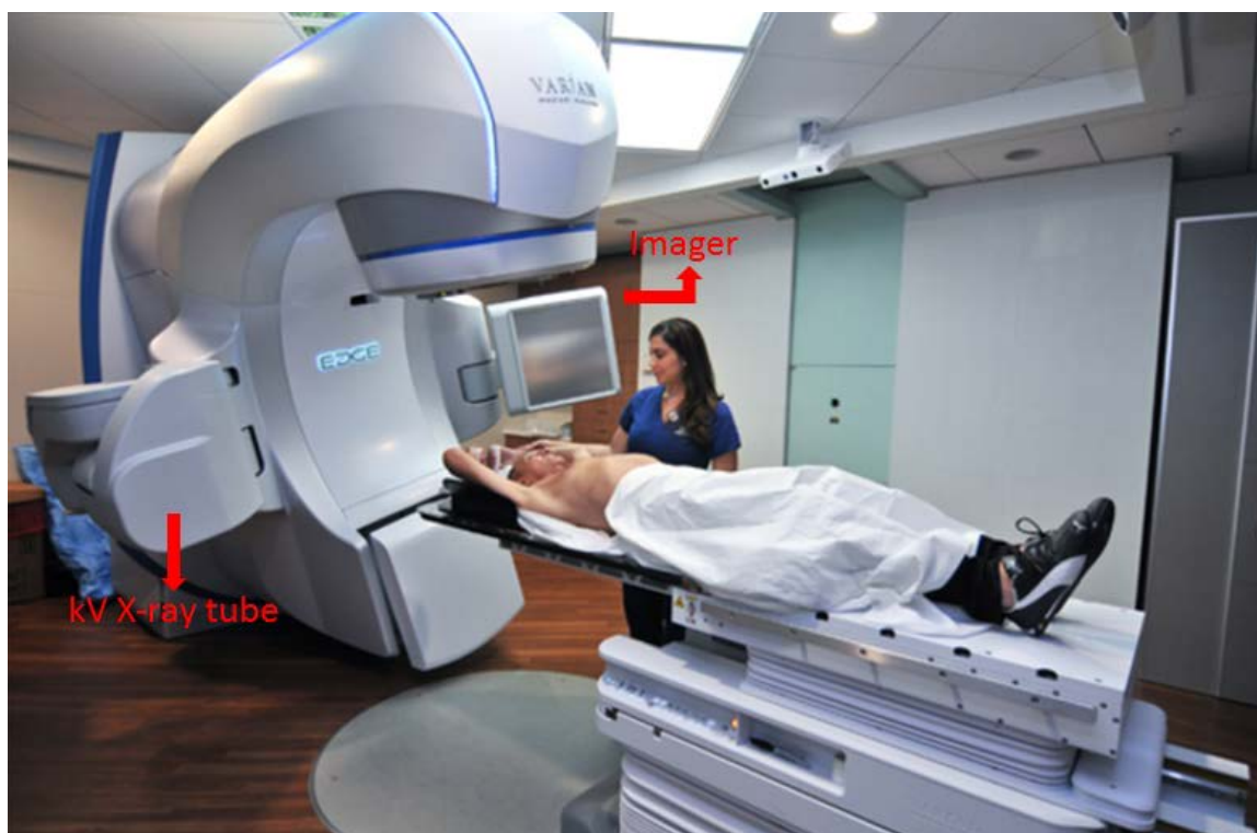
Figure. 1.11 A photo of Varian Edge ® LINAC with OBI marked at Innovative Cancer Institute (South Miami, FL). The kV X-ray tube and imager are marked in red. They are folding back to standby position.
