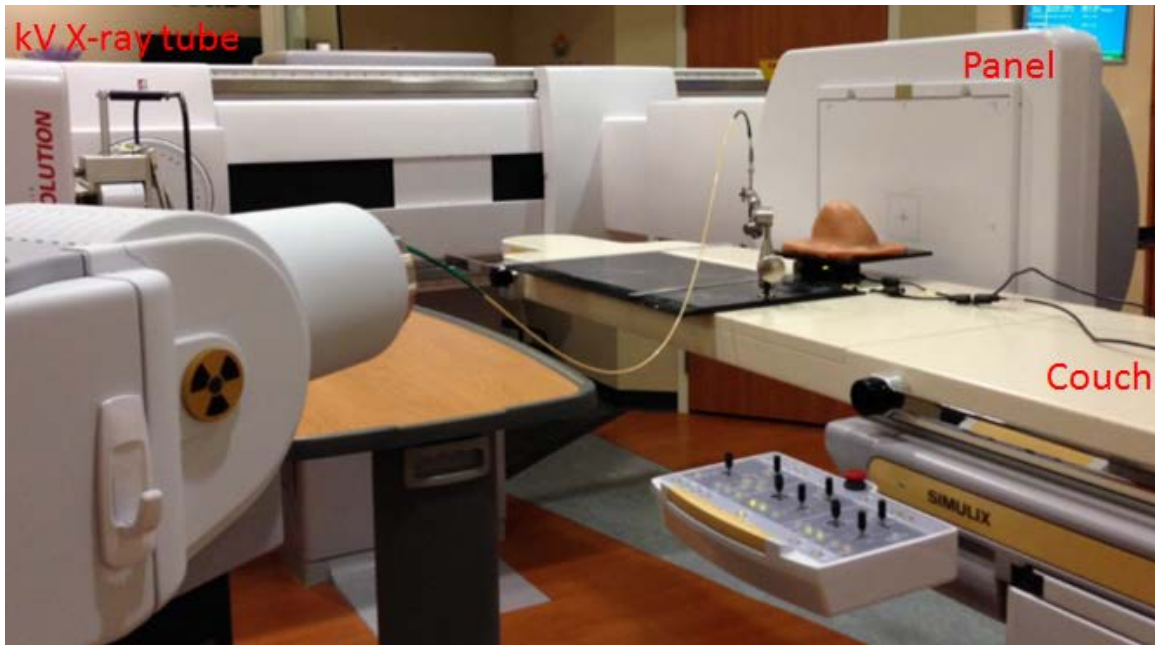
Figure 3.7 Simulix Evolution brachytherapy CT simulator. We rotated the gantry 90 degrees to the horizontal position in this figure, so the surface of the detector was parallel to the surface of the collimator.
