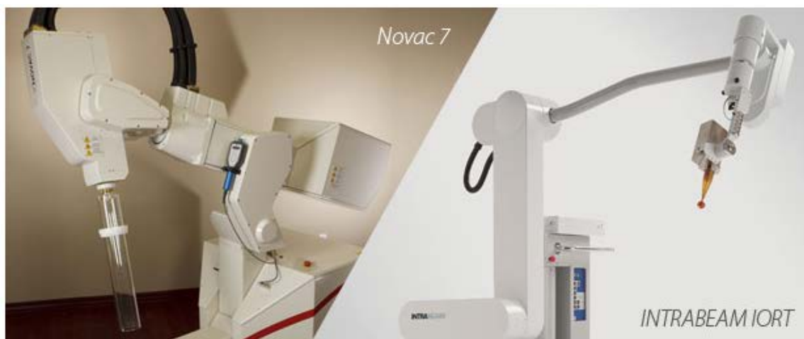
Figure 1.17 Mobile IORT devices. Left: Novac 7 (New Radiant Technology – NRT, Rome, Italy), a Electron IORT device, can generate 4, 6, 8 and 10 MeV electron beams. Right: INTRABEAM (ZEISS, Oberkochen, Germany), a low-energy X-rays device, provides 50 kV photon beams.
