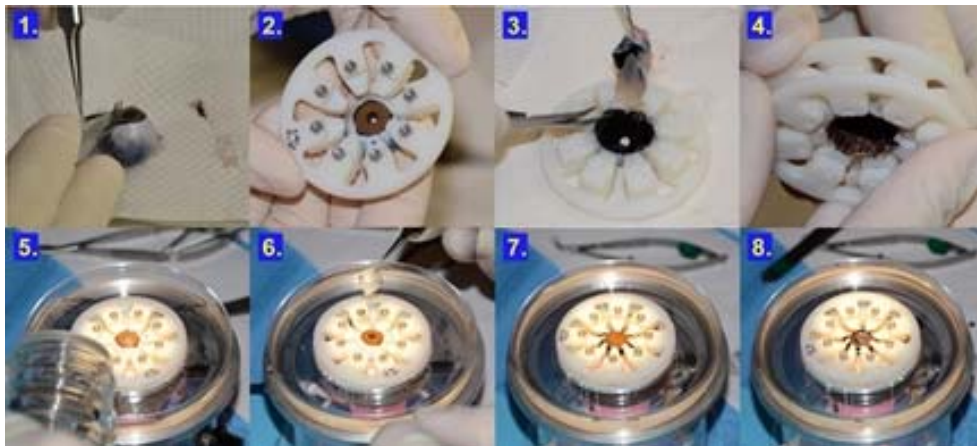
Figure 3.2: EVAS II tissue dissection procedure. 1) The extraocular muscles were removed, 2) then the equatorial globe diameter was measured with digital calipers and the best-fitting shoe size was selected. Cyanoacrylate glue was applied to the individual shoes and the eye was aligned and mounted onto the shoes. Once the glue dried, 3) the posterior pole was removed, and 4) the bottom retaining ring was added. 5) The tissue was transferred to a Petri dish atop a custom-made portable dissection stage with diffuse retro-illumination and Dulbecco's modified Eagle's medium was added to preserve the tissue. 6) The cornea was removed and 7) the scleral segments were excised. 8) Lastly, the iris was removed and the tissue is ready to be transferred into the EVAS II system (Nankivil et al. 2015).
