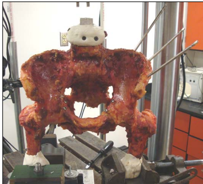
Figure 11: Final test model, double leg stance.
