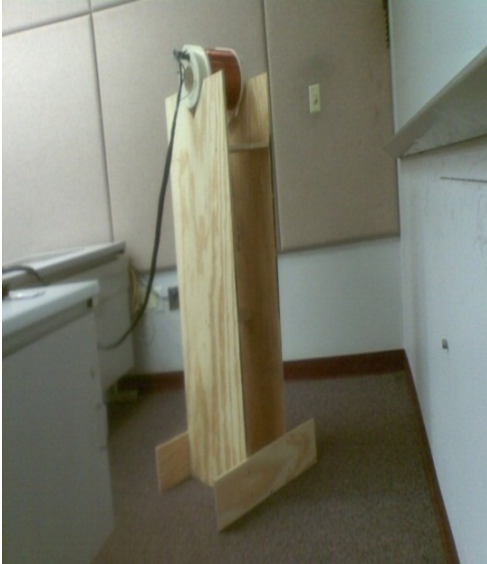
Figure 3. 8 The wooden stand that supports the probe.
