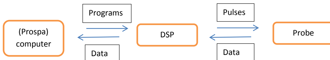
Figure 3.4 The flow chart describes the whole working process of the EFNMR system.
