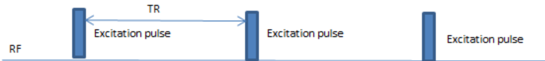
Figure 2. 10 Time of repeat (TR) is the duration interval between two RF pulses.
