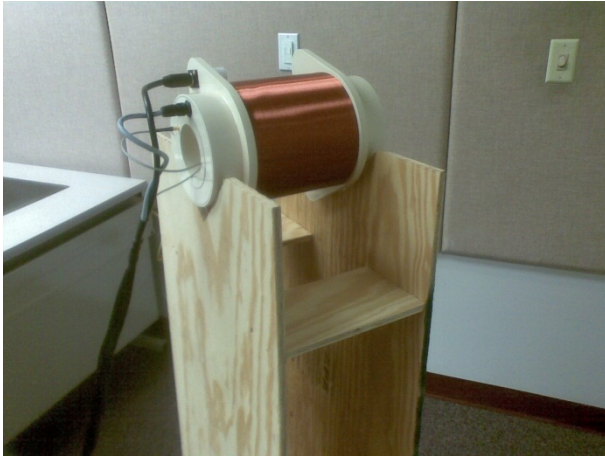
Figure 3.1 The probe used in the experiment. It consists of three sets of coil.
