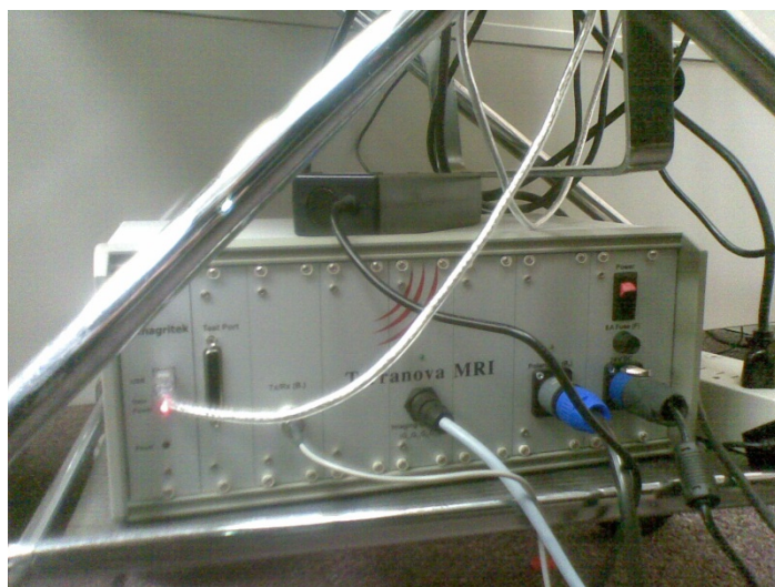
Figure 3. 3 The digital signal processor. It controls the probe.
