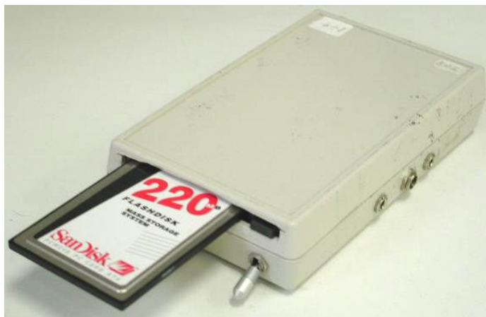
Figure 4.3 Battery powered data-logging device for recording two channels of EMG at 3200 Hz. The device stores the data on a type II PCMCIA flashcard or compactflash card, which acts as a hard disk drive.
