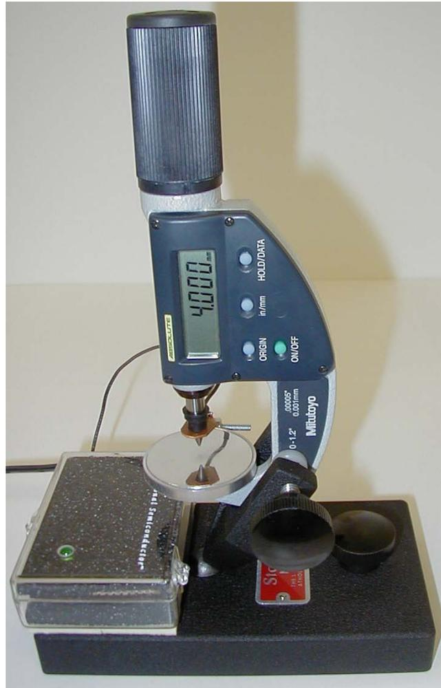
**Figure 3-4: Photograph of the current sensing micrometer**
