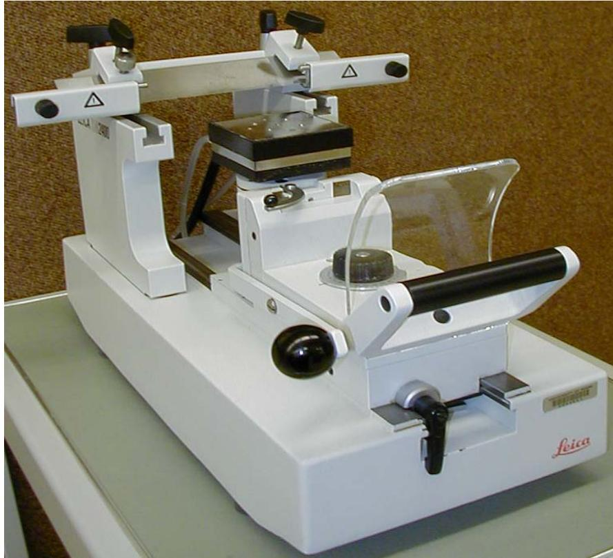
**Figure 3-3: Photograph of the sledge microtome with freezing stage**
