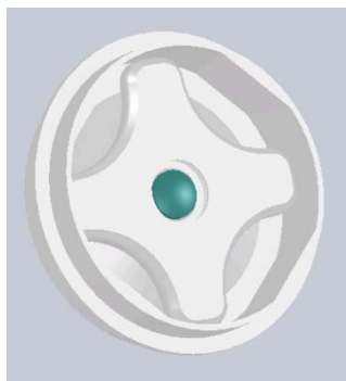
Figure 3.1: SolidWorks Rendition of the Custom Corneal Holder with the Anchoring Top and the Base Assembled.
