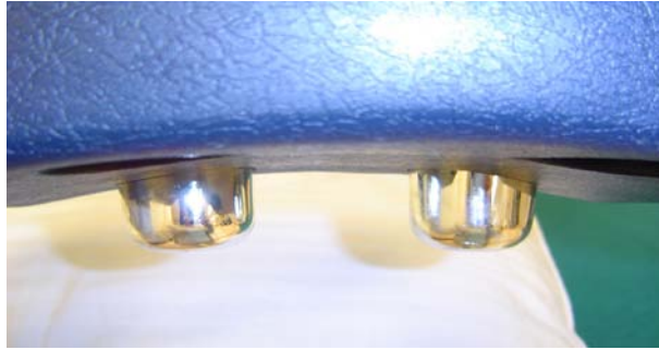
Figure 2.2: Hand-held vibrator. This device (Pro-Massager USJ-301, U.S. Jaclean, Inc. Gardena, CA, USA) was used to deliver vibration to target a specific leg muscle. The vibration was given at the frequency of 60 Hz with an unloaded amplitude of approximately 1 mm.
