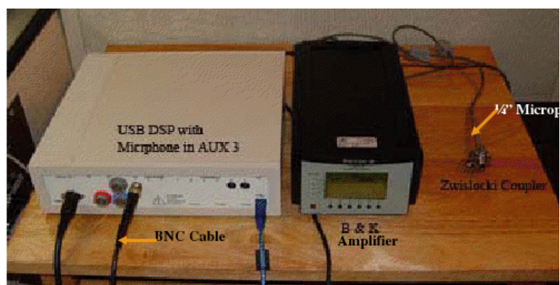
Figure 2.2.2 – Calibration setup, consisting of an IHS USB System, a B&K microphone conditioning amplifier, and a B&K calibration microphone with a Zwislocki coupler. Courtesy of Intelligent Hearing Systems (IHS)
