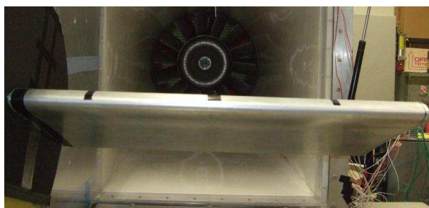
Figure 2.15: Downstream View of Model Mounted in Test Section
