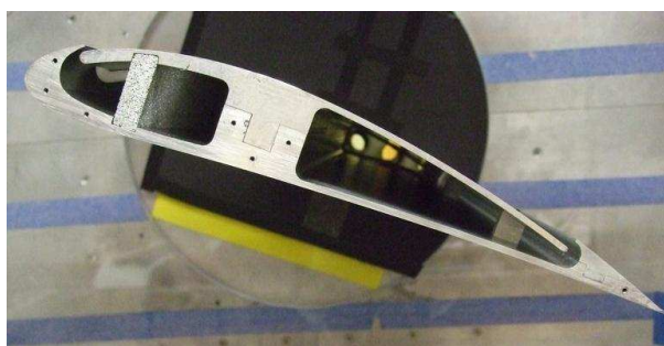
Figure 2.13: Cavities of Manufactured CFJ Airfoil
