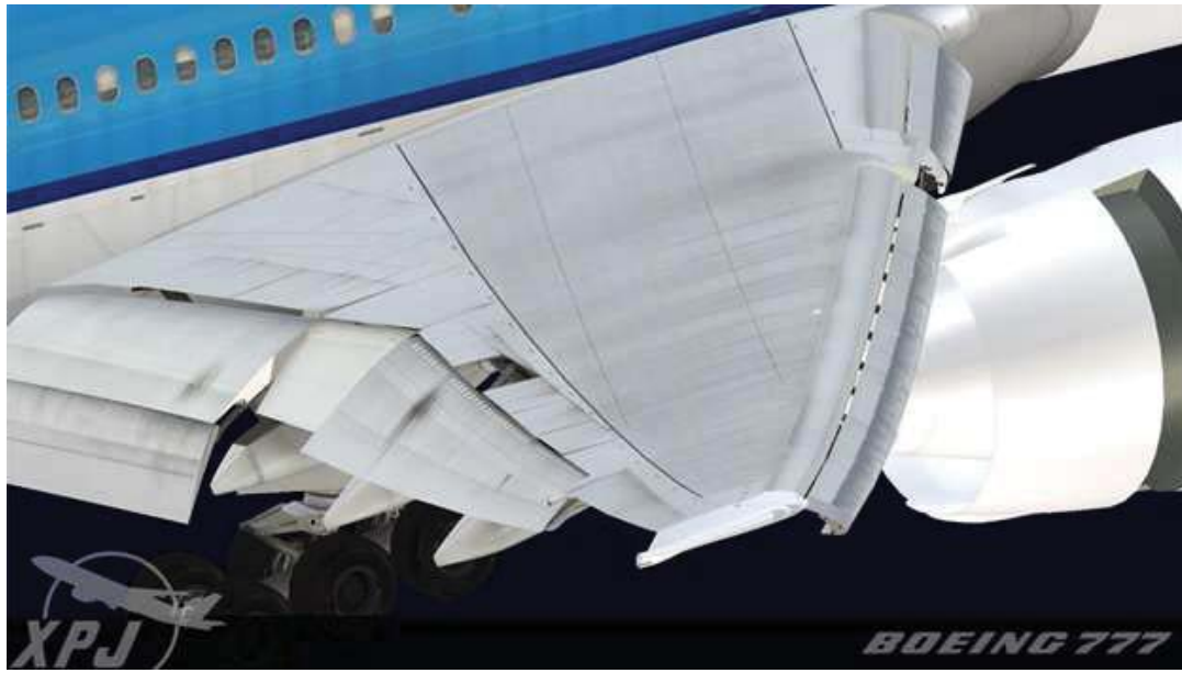
Figure 1.5: Boeing 777 at takeoff with flaps and slats fully deployed. Notice the vortex generators located on the outboard flap. Credit: Boeing.
