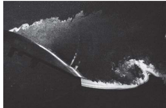
Figure 1.11: Massive flow separation of baseline NACA 6415 airfoil at AoA=25^\circ .
